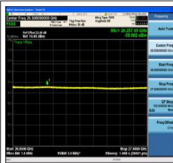
1-N77-3700-3980-PC2-30-40-M-15-DFT-256 QAM-Outer_Full-100@0-26000-40000-Ant1-- 33.58--13-PASS
