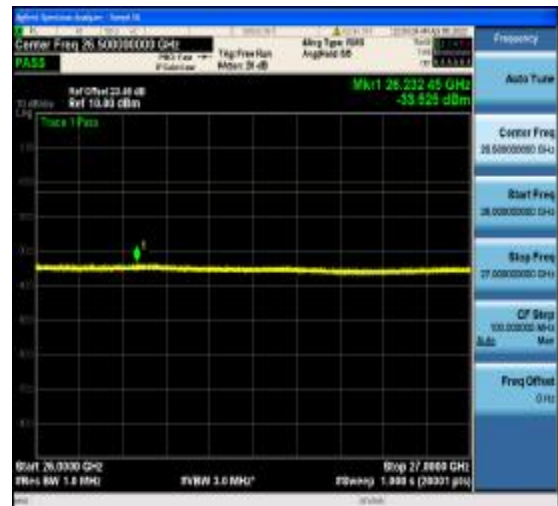
1-N77-3700-3980-PC2-30-40-M-20-CP-16Q AM-Edge_1RB_Right-1@105-26000-40000- Ant1--33.52--13-PASS
