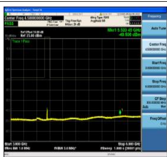
1-N77-3700-3980-PC2-30-40-M-20-CP-16Q AM-Edge_1RB_Right-1@105-3000-6000-Ant 1--49.51--13-PASS
