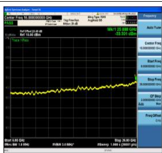
1-N77-3700-3980-PC2-30-80-L-10-DFT-64Q AM-Edge_1RB_Left-1@0-6000-26000-Ant1-- 33.30--13-PASS
