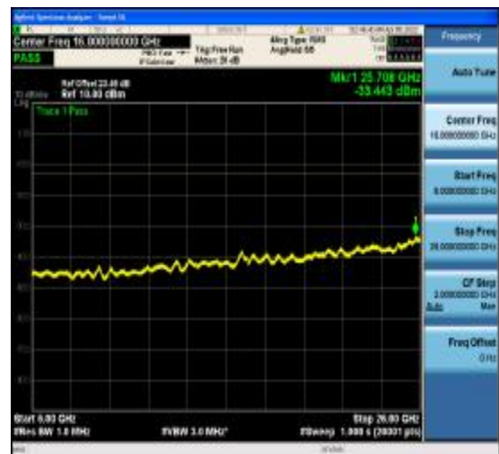
1-N77-3700-3980-PC2-30-60-M-22-CP-64Q AM-Edge_1RB_Left-1@0-6000-26000-Ant1-- 33.44--13-PASS
