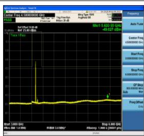
1-N77-3700-3980-PC2-30-80-L-13-DFT-256 QAM-Edge_1RB_Left-1@0-3000-6000-Ant1- -49.03--13-PASS
