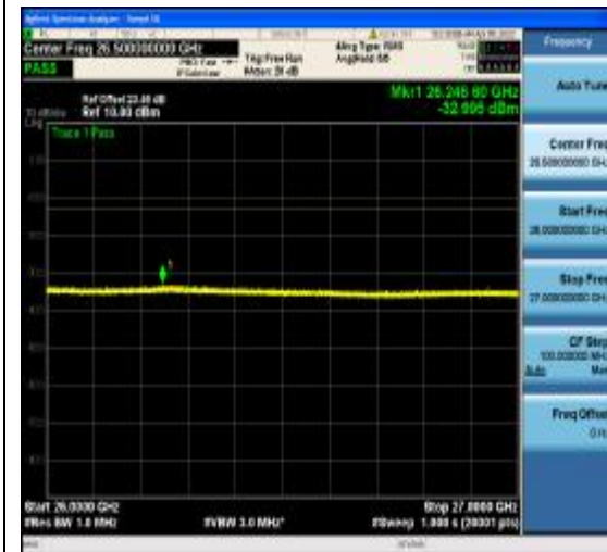
1-N77-3700-3980-PC2-30-60-H-17-CP-QPS K-Edge_1RB_Right-1@161-26000-40000-An t1--32.99--13-PASS
