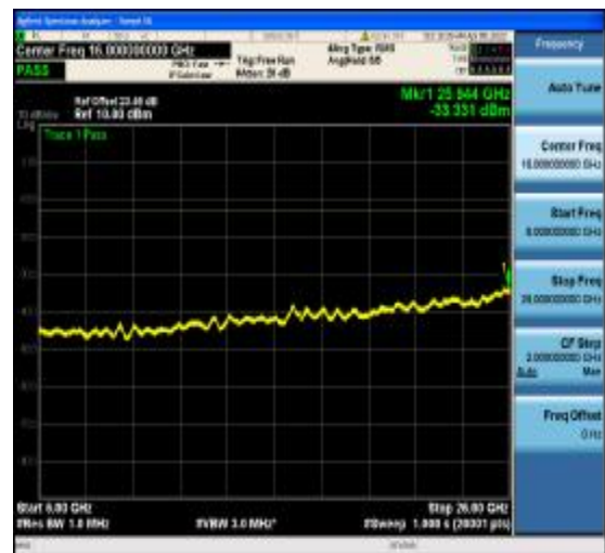
1-N77-3700-3980-PC2-30-60-H-7-DFT-16QA M-Edge_1RB_Left-1@0-6000-26000-Ant1--3 3.33--13-PASS
