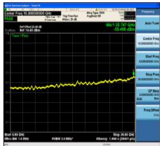
1-N77-3700-3980-PC2-30-60-M-26-CP-256Q AM-Edge_1RB_Right-1@161-6000-26000-A nt1--33.46--13-PASS
