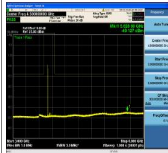
1-N77-3700-3980-PC2-30-80-M-25-CP-256Q AM-Edge_1RB_Left-1@0-3000-6000-Ant1--4 9.13--13-PASS
