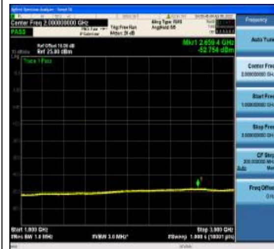
1-N77-3700-3980-PC2-30-80-M-4-DFT-QPS K-Edge_1RB_Left-1@0-1000-3000-Ant1--52. 75--13-PASS
