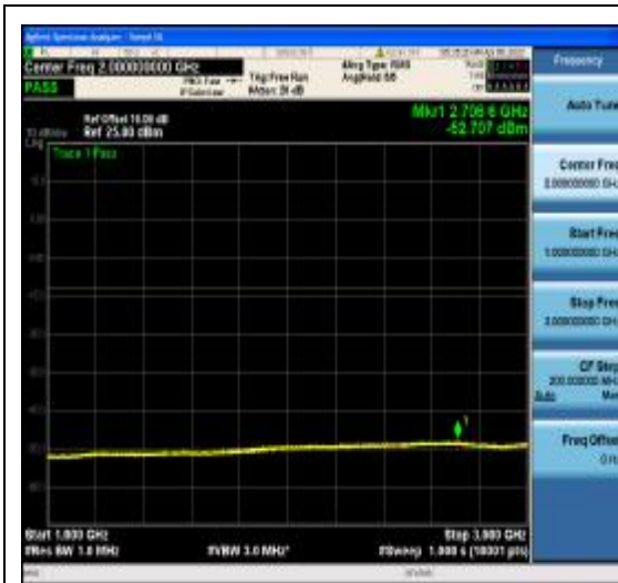
1-N77-3700-3980-PC2-30-80-M-22-CP-64Q AM-Edge_1RB_Left-1@0-1000-3000-Ant1--5 2.71--13-PASS
