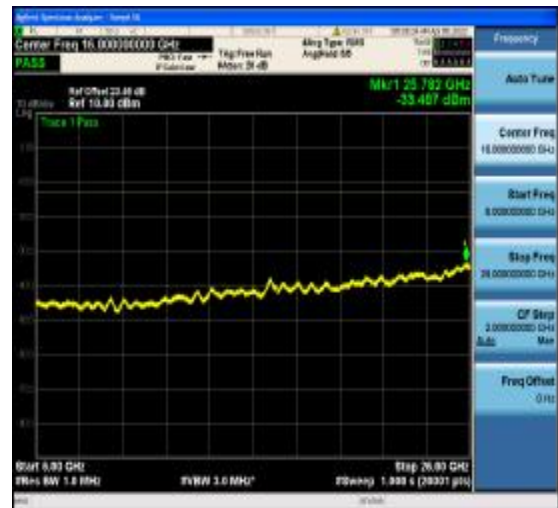
1-N77-3700-3980-PC2-30-80-M-13-DFT-256 QAM-Edge_1RB_Left-1@0-6000-26000-Ant1 --33.49--13-PASS
