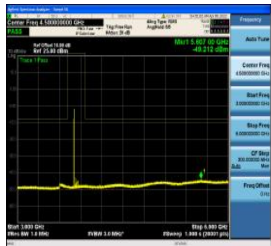
1-N77-3700-3980-PC2-30-80-M-4-DFT-QPS K-Edge_1RB_Left-1@0-3000-6000-Ant1--49. 21--13-PASS
