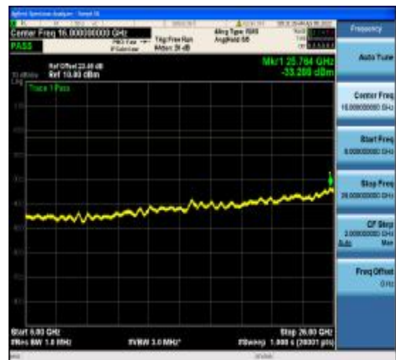
1-N77-3700-3980-PC2-30-80-M-25-CP-256Q AM-Edge_1RB_Left-1@0-6000-26000-Ant1-- 33.29--13-PASS
