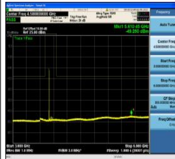
1-N77-3700-3980-PC2-30-80-M-13-DFT-256 QAM-Edge_1RB_Left-1@0-3000-6000-Ant1- -49.25--13-PASS
