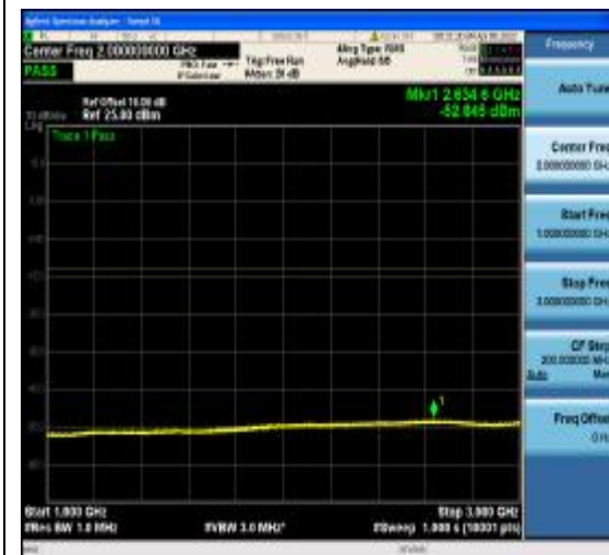
1-N77-3700-3980-PC2-30-80-M-20-CP-16Q AM-Edge_1RB_Right-1@216-1000-3000-Ant 1--52.84--13-PASS
