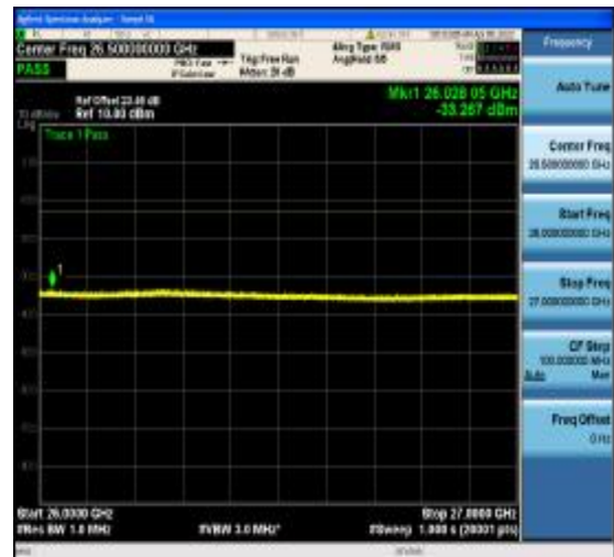
1-N77-3700-3980-PC2-30-80-M-10-DFT-64Q AM-Edge_1RB_Left-1@0-26000-40000-Ant1 --33.27--13-PASS
