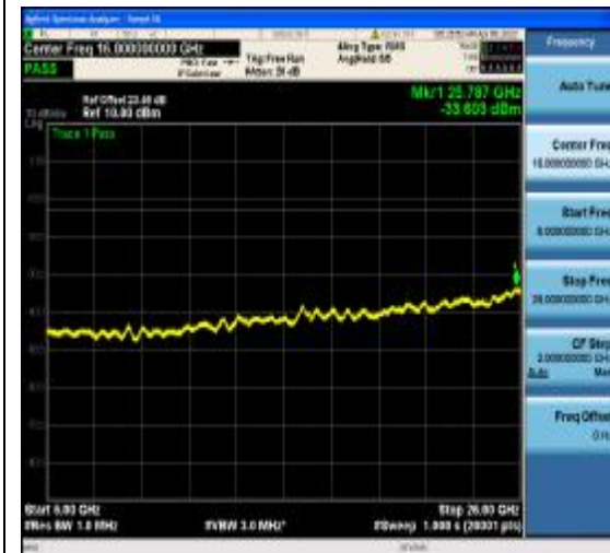
1-N77-3700-3980-PC2-30-80-M-22-CP-64Q AM-Edge_1RB_Left-1@0-6000-26000-Ant1-- 33.60--13-PASS
