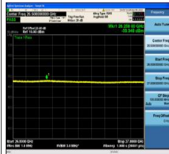
1-N77-3700-3980-PC2-30-80-M-7-DFT-16QA M-Edge_1RB_Left-1@0-26000-40000-Ant1-- 33.35--13-PASS
