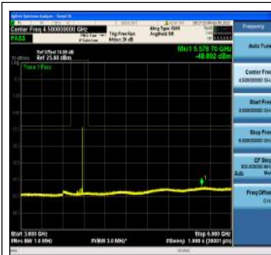
1-N77-3700-3980-PC2-30-80-M-23-CP-64Q AM-Edge_1RB_Right-1@216-3000-6000-Ant 1--48.89--13-PASS
