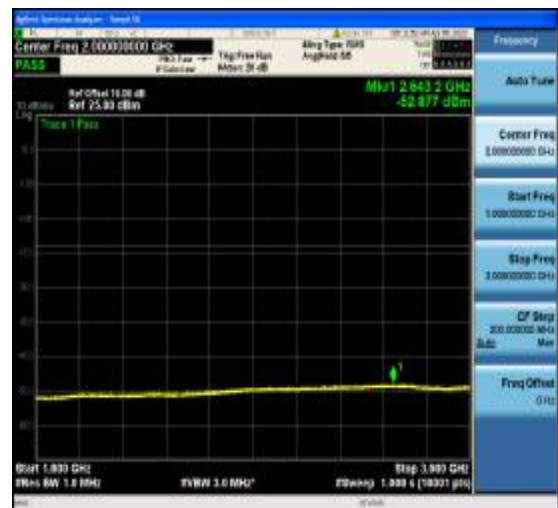
1-N77-3700-3980-PC2-30-80-M-15-DFT-256 QAM-Outer_Full-216@0-1000-3000-Ant1--52 .88--13-PASS
