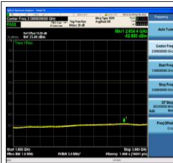
1-N77-3700-3980-PC2-30-80-M-10-DFT-64Q AM-Edge_1RB_Left-1@0-1000-3000-Ant1--5 2.88--13-PASS
