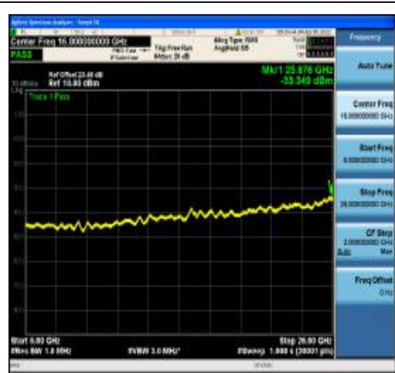
1-N77-3700-3980-PC2-30-80-M-11-DFT-64Q AM-Edge_1RB_Right-1@216-6000-26000-A nt1--33.35--13-PASS
