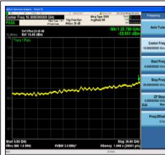
1-N77-3700-3980-PC2-30-80-L-15-DFT-256 QAM-Outer_Full-216@0-6000-26000-Ant1--3 3.55--13-PASS
