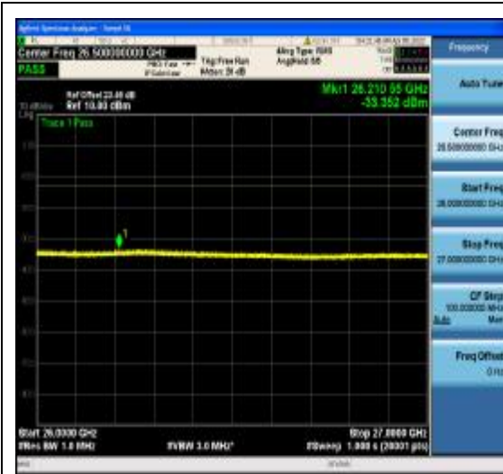
1-N77-3700-3980-PC2-30-80-L-16-CP-QPSK -Edge_1RB_Left-1@0-26000-40000-Ant1--3 3.35--13-PASS
