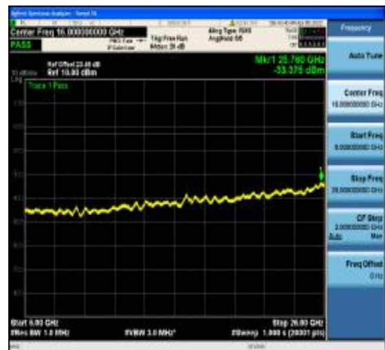
1-N77-3700-3980-PC2-30-100-L-7-DFT-16Q AM-Edge_1RB_Left-1@0-6000-26000-Ant1-- 33.38--13-PASS
