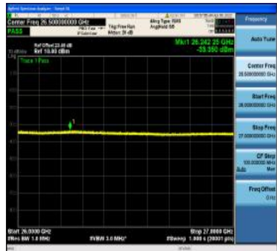
1-N77-3700-3980-PC2-30-80-H-11-DFT-64Q AM-Edge_1RB_Right-1@216-26000-40000- Ant1--33.35--13-PASS
