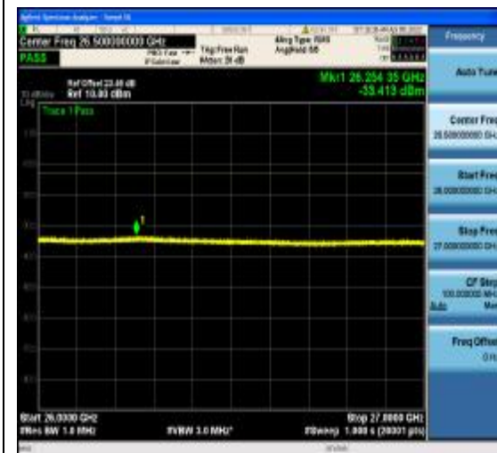
1-N77-3700-3980-PC2-30-100-L-25-CP-256 QAM-Edge_1RB_Left-1@0-26000-40000-Ant 1--33.41--13-PASS
