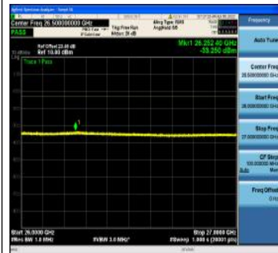
1-N77-3700-3980-PC2-30-100-M-2-DFT-PI2 BPSK-Edge_1RB_Right-1@272-26000-4000 0-Ant1--33.25--13-PASS
