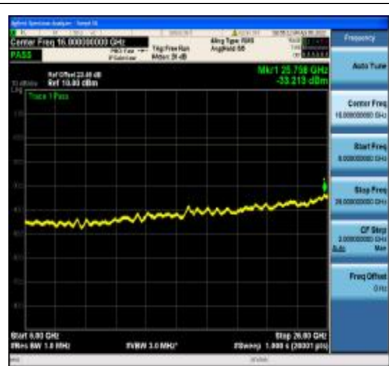
1-N77-3700-3980-PC2-30-100-L-13-DFT-256 QAM-Edge_1RB_Left-1@0-6000-26000-Ant1 --33.21--13-PASS
