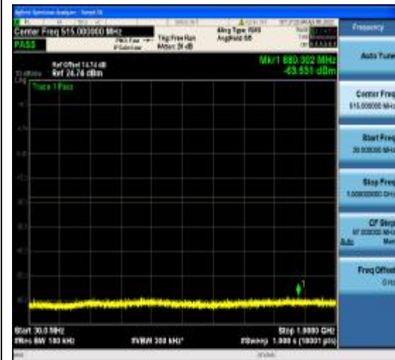
1-N77-3700-3980-PC2-30-100-L-25-CP-256 QAM-Edge_1RB_Left-1@0-30-1000-Ant1--6 3.53--23-PASS
