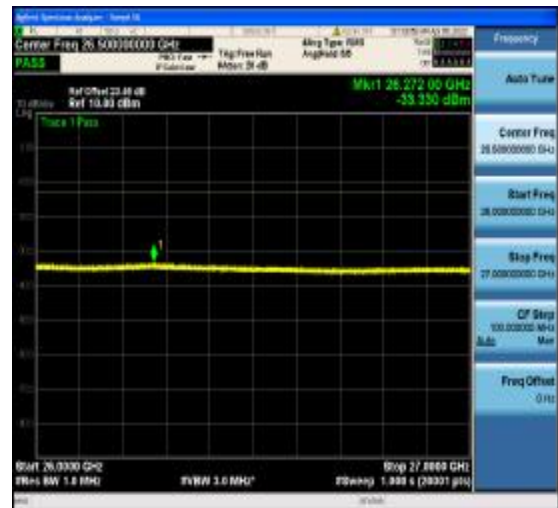
1-N77-3700-3980-PC2-30-100-L-20-CP-16Q AM-Edge_1RB_Right-1@272-26000-40000- Ant1--33.33--13-PASS
