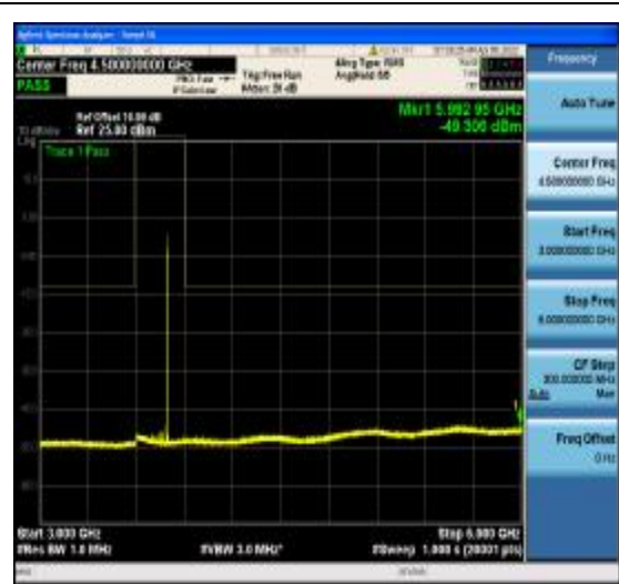
1-N77-3700-3980-PC2-30-100-L-20-CP-16Q AM-Edge_1RB_Right-1@272-3000-6000-Ant 1--49.31--13-PASS
