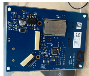
Endpoint (LoRa) Board w/trace antenna
