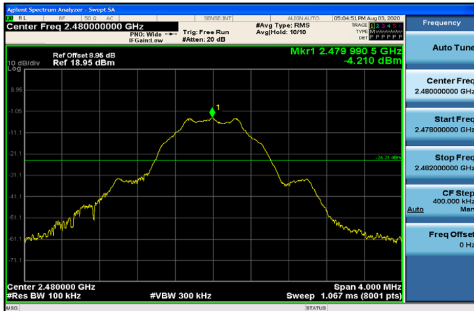
RF Conducted Spurious Emissions_BLE_2480_1M
