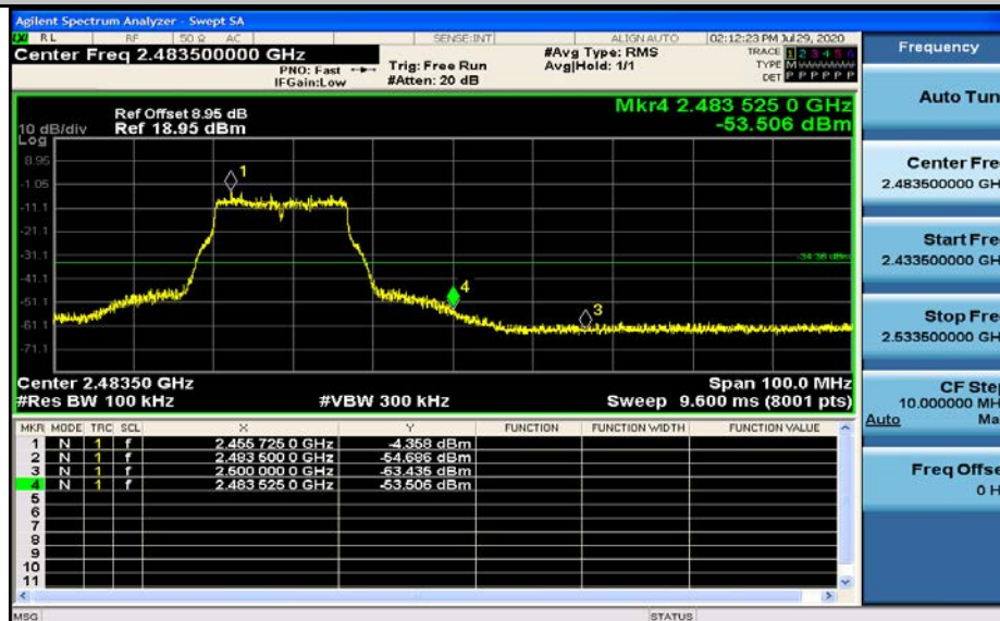
Band-edge for RF Conducted Emissions_11N20SISO_2412_Ant1
