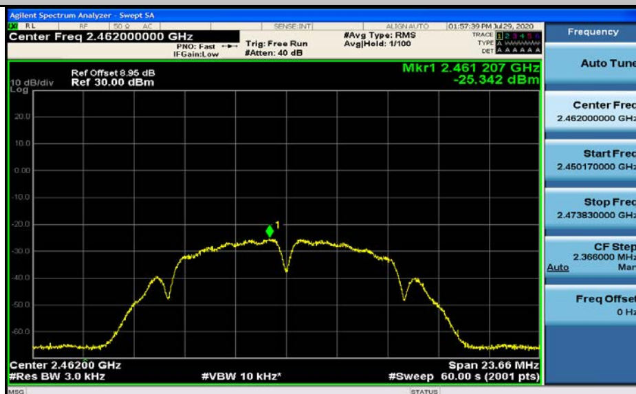
Maximum(average) power spectral density_11B_2462_Ant1
