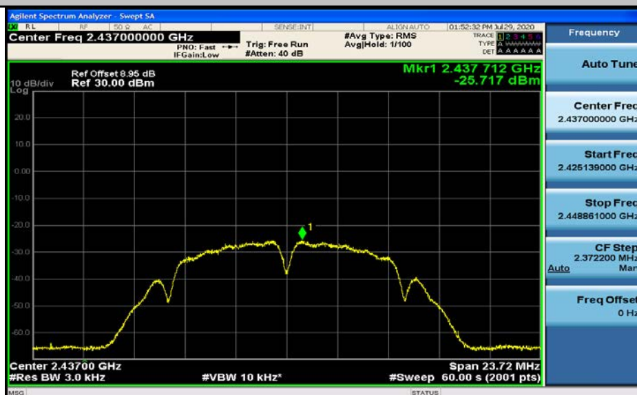
Maximum(average) power spectral density_11B_2462_Ant1
