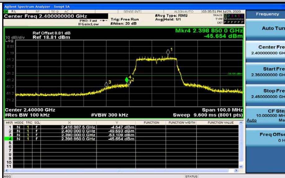
Band-edge for RF Conducted Emissions_11N20SISO_2462_Ant1
