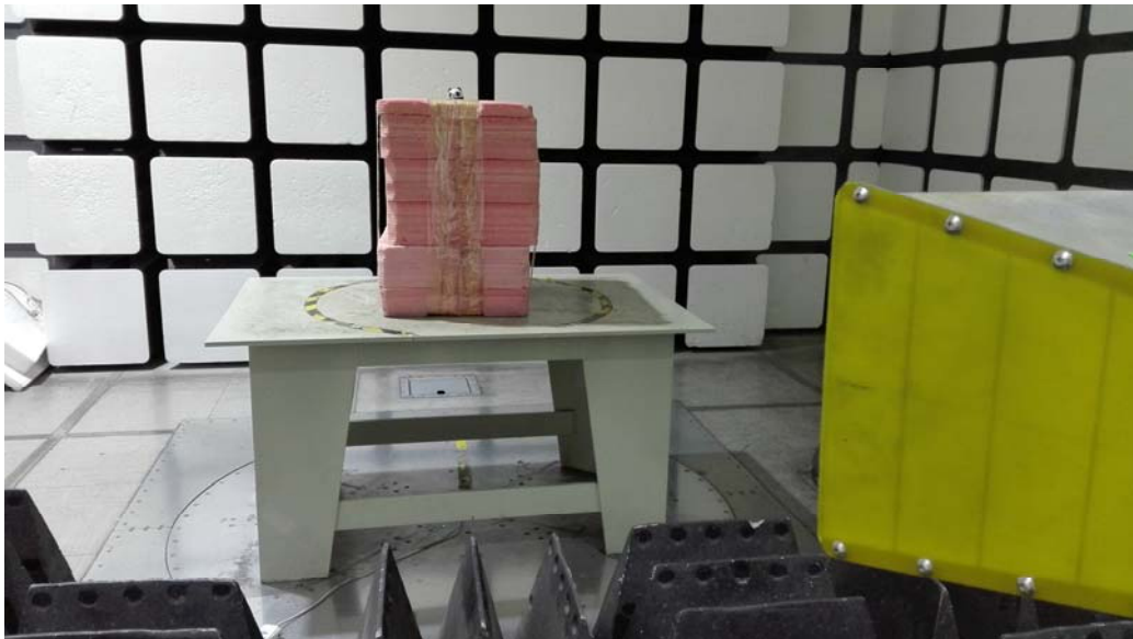
Radiated Emissions View (Above 1 GHz)
