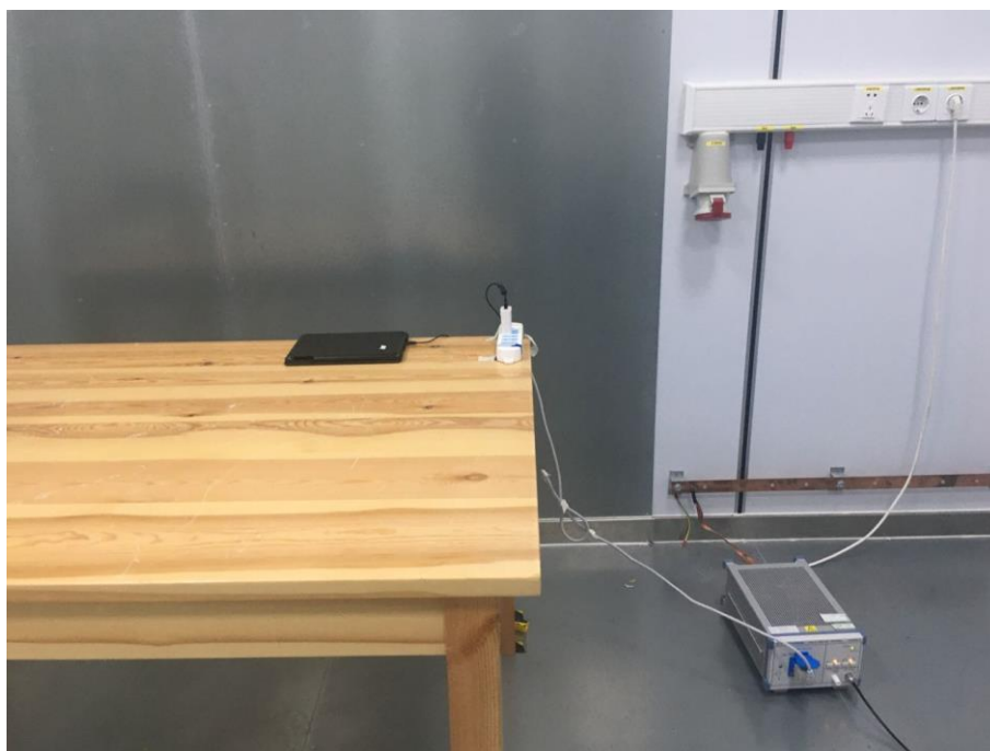
Fig. 5 AC Power Line Conducted emission setup photo
