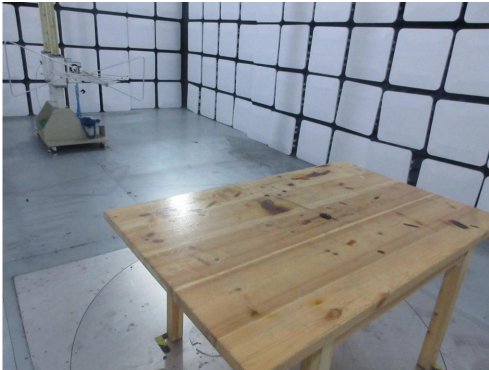
FCC ID: 2ACAL-ABCONN06 Photo of Radiation Emission Test
