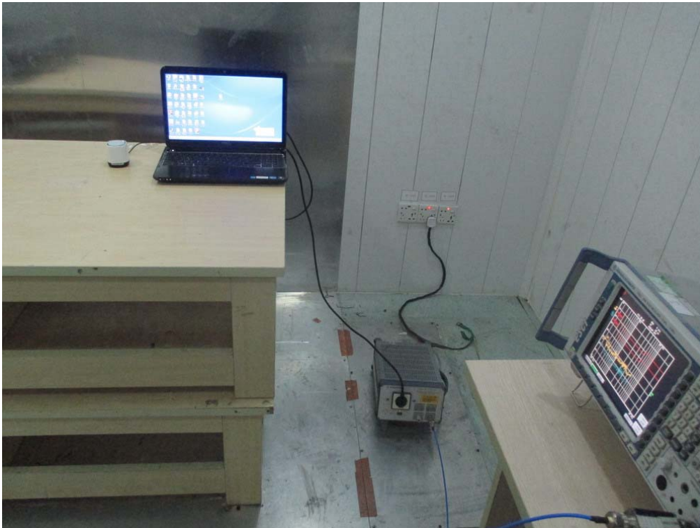
FCC RADIATED EMISSION TEST SETUP
