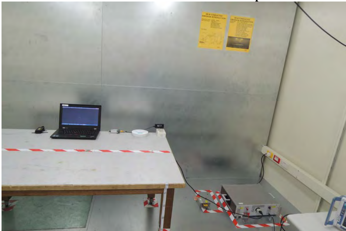
AC Power-line Conducted Emission Set up Photo
