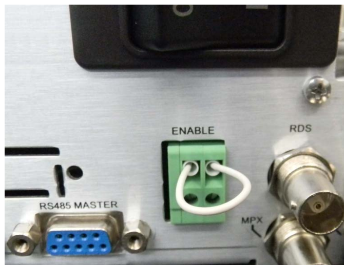
Fig. 8 – ENABLE short circuit (INTERLOCK)
