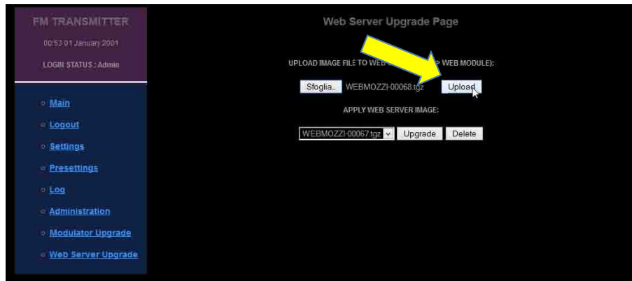
Fig. 8.20 – Upload the firmware to webserver
