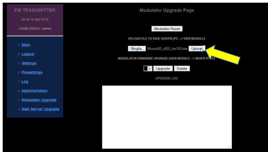
Fig. 8.12 – Upload the new firmware
