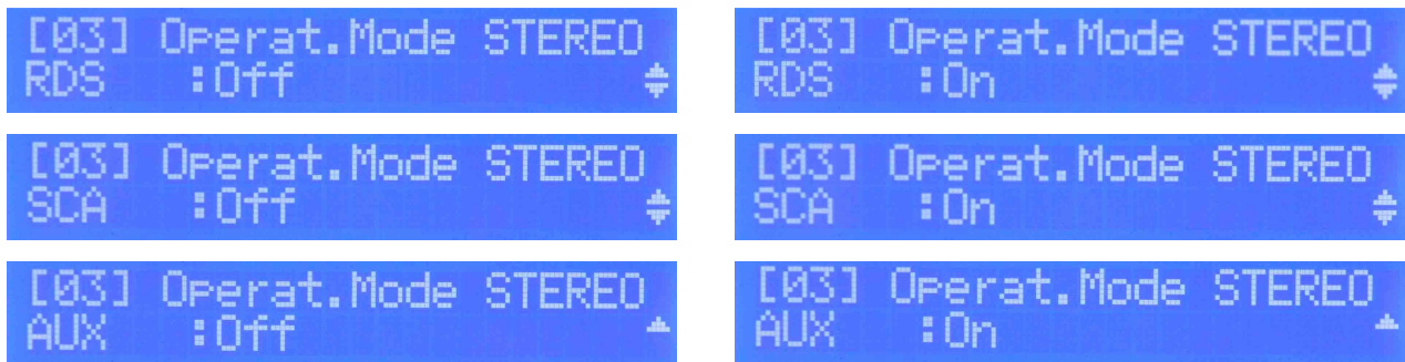
Fig. 5.19 – Auxiliary channels options
