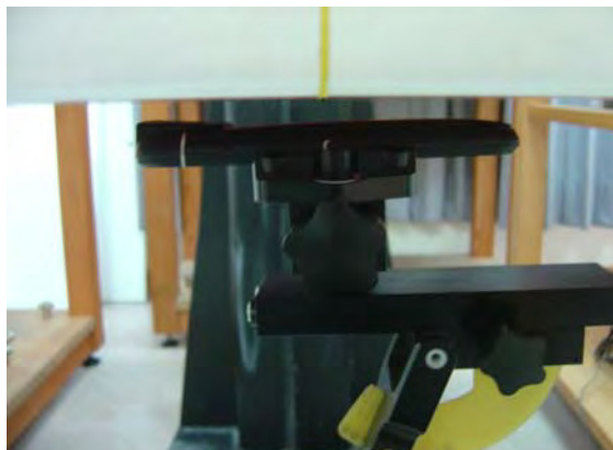
Fig.8 EUT back to flat phantom
