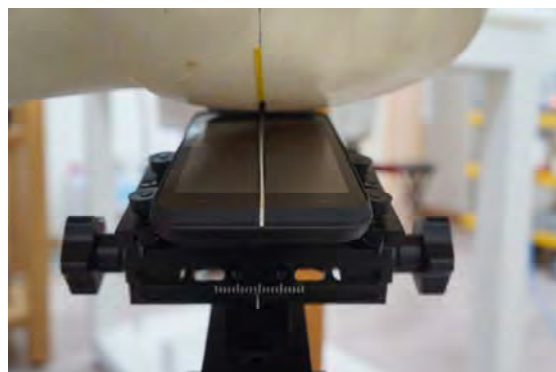
Fig.6 Left Head Section / Ear-Tilt Position(15°)
