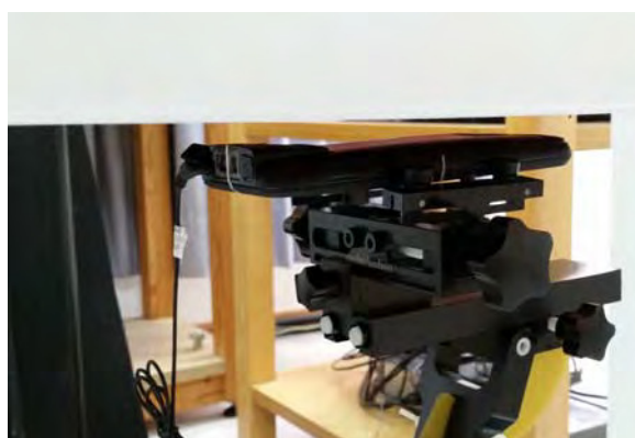
Fig.14 EUT back with headset to flat phantom
