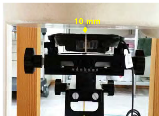
Fig.13 EUT front with headset to flat phantom
