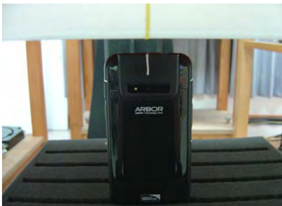
Fig.9 EUT top to flat phantom
