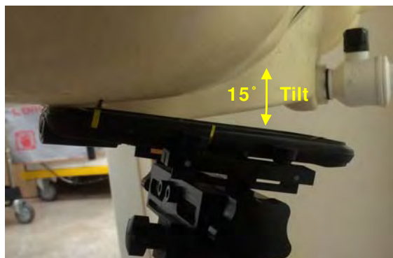
Fig.3 Right Head Section / Cheek-Touch Position
