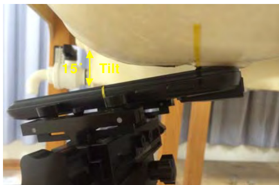
Fig.6 Left Head Section / Ear-Tilt Position(15°)
