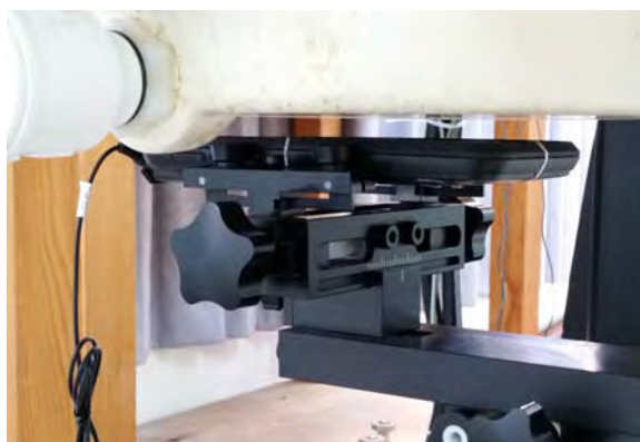
Fig.13 EUT front with headset to flat phantom
