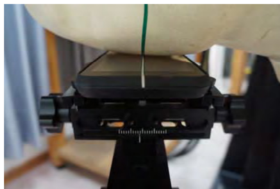
Fig.3 Right Head Section / Cheek-Touch Position
