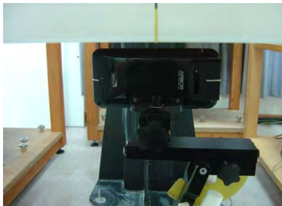
Fig.11 EUT right to flat phantom
