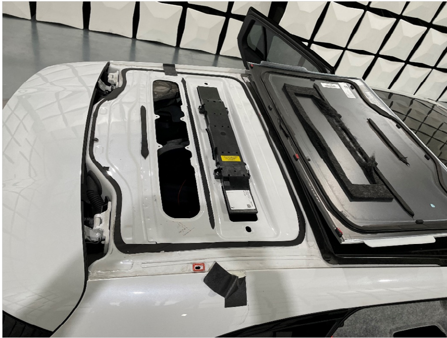
Photograph 3: AE 2 (Antenna placement)
