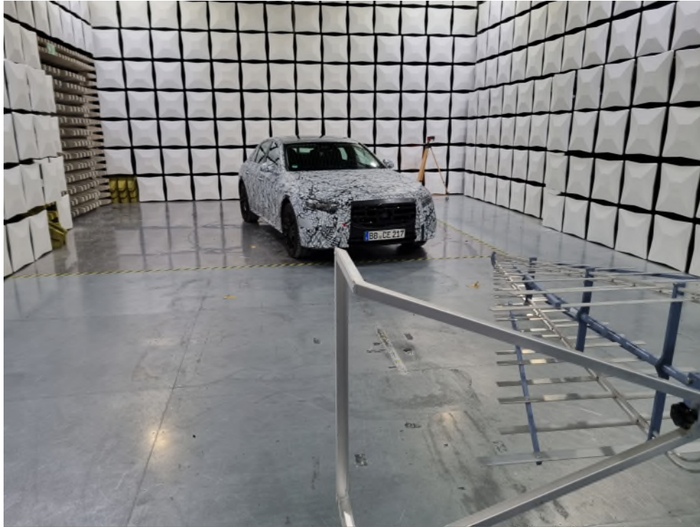
Fig. 5: Set up with EUT for test without absorbers at a car (E-Class (W214))
