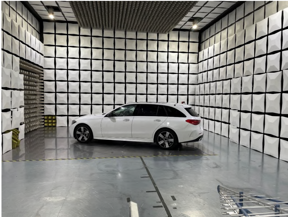
Fig. 5: Set up with EUT for test without absorbers at a car (C-Class station wagon (S206)).
