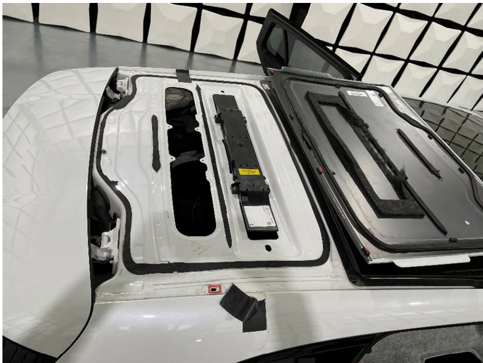
Fig. 6: EUT support details: set up when measuring the real antenna installed at the car (but cover removed).
