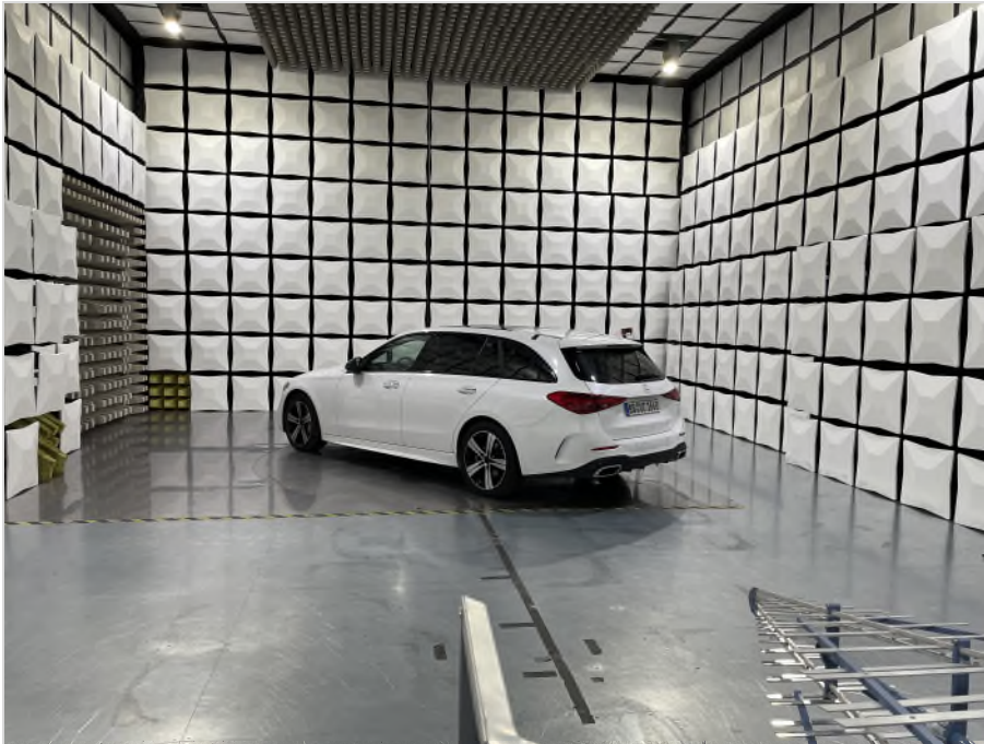
Photograph 1: EUT Test Setup in the anechoic chamber, Radiated interference field strength (frequency range below 1GHz)
