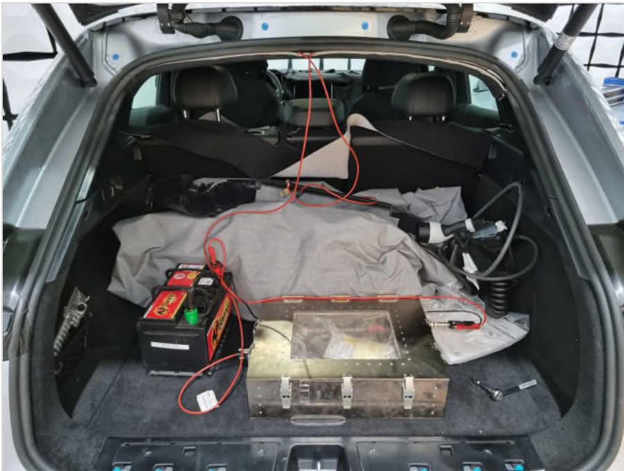
Photograph 4: Placement AE1 inside shielded enclosure
