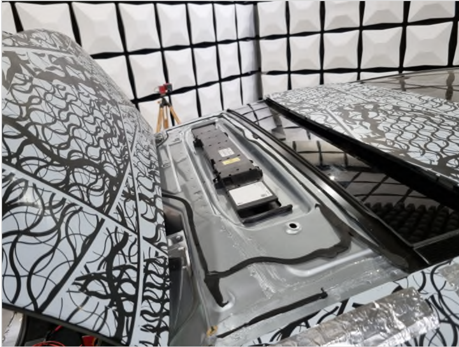
Photograph 3: EUT test setup in the anechoic chamber, close up view on EUT placement
