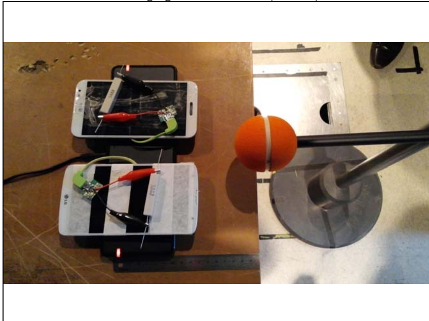
Charging Mode with load (E-Field)
