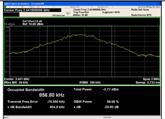
GFSK - Middle Channel
