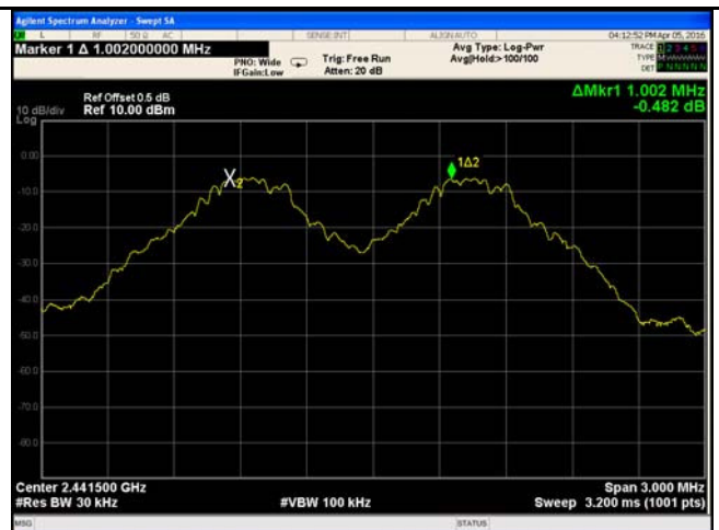
GFSK - Middle Channel
