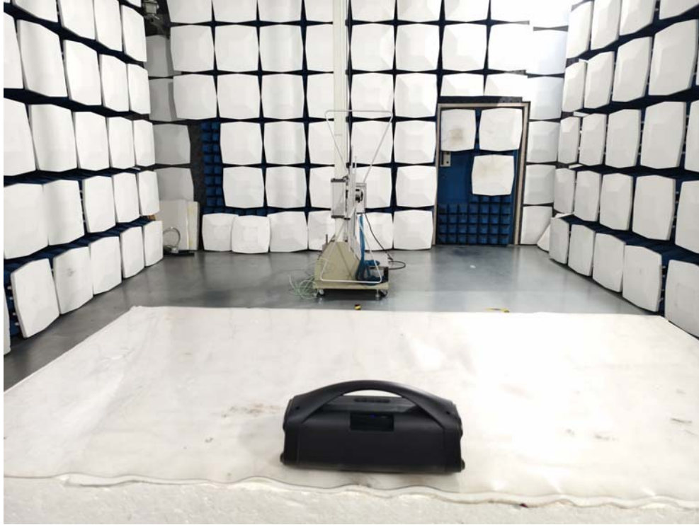
Radiated Emission Test Setup:
