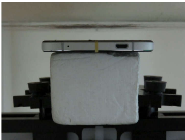
Back, Test Separation 10 mm
