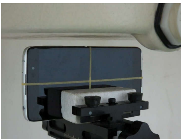
Right Side, Test Separation 10 mm
