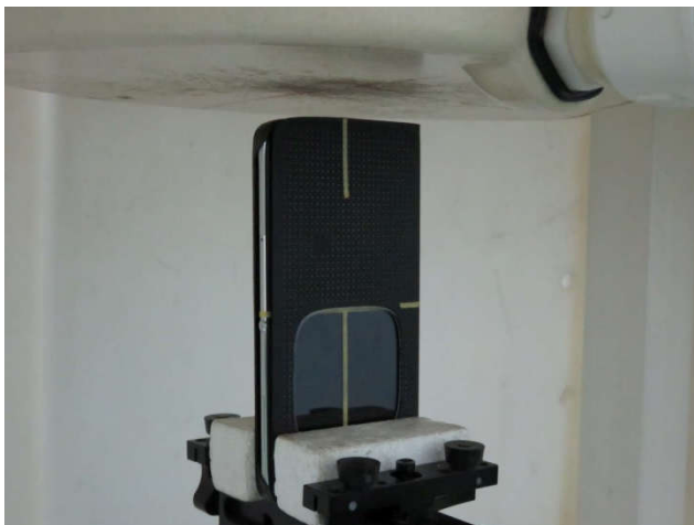
Bottom Side, Test Separation 10 mm
