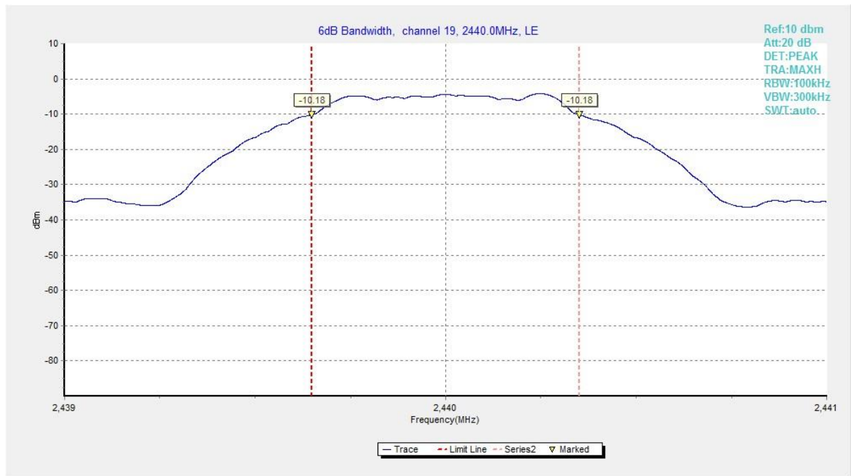
Fig.5 6dB Bandwidth (Ch 19), LE 1M
