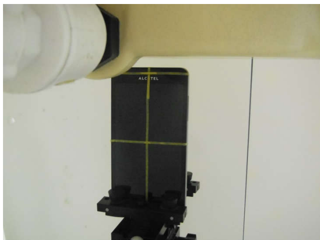
Top Side, Test Separation 10 mm
