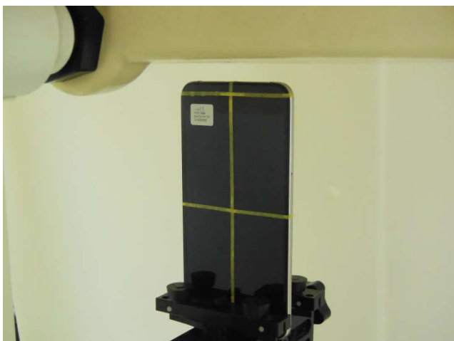
Top Side, Test Separation 10 mm
