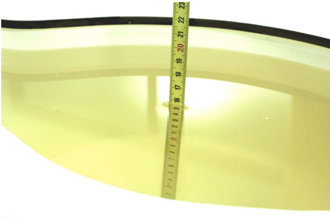
Picture 7-12 Liquid depth in the Flat Phantom (2600MHz)
