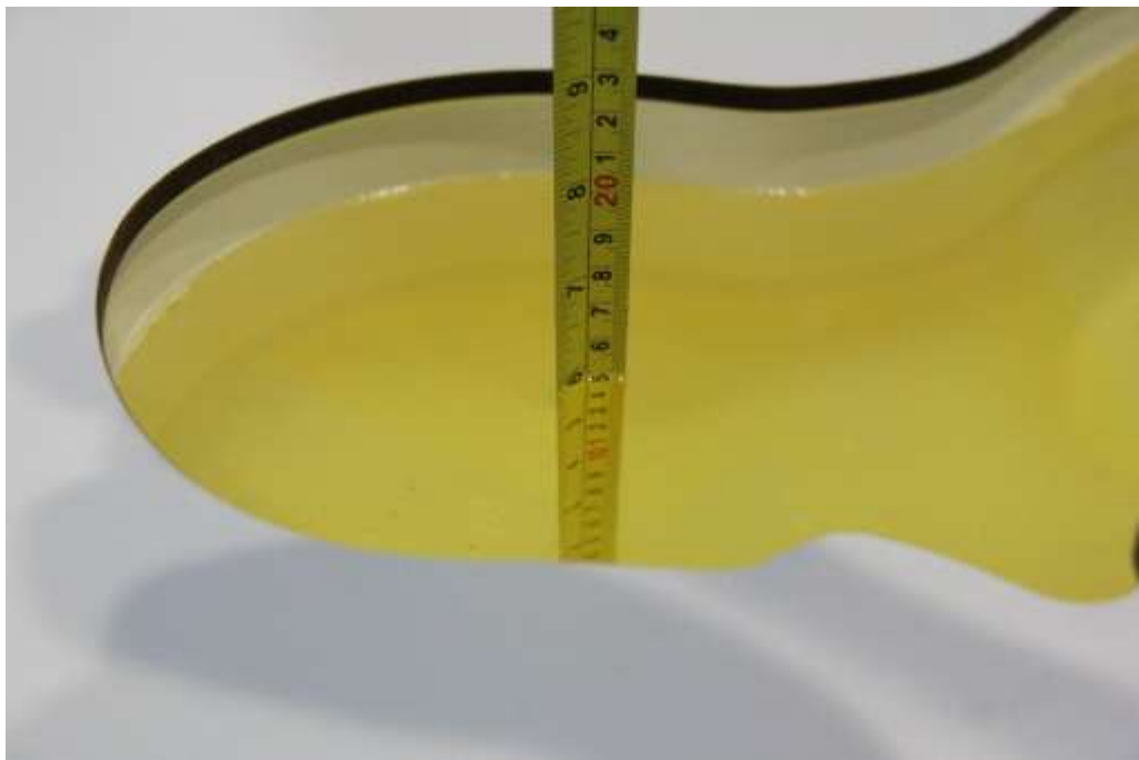
Picture 7-4: Liquid depth in the Head Phantom(2450MHz)
