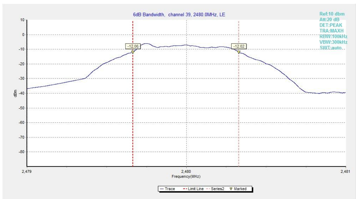
Fig.6 6dB Bandwidth (Ch 39), LE 1M
