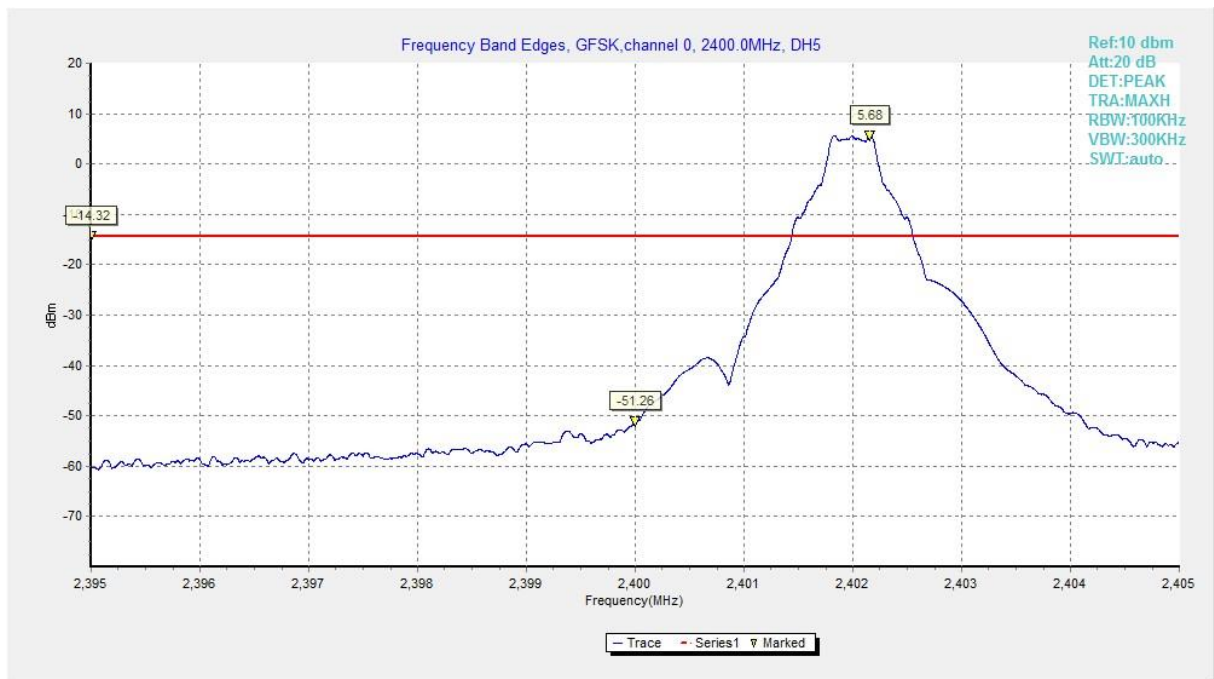
Fig. 7 Band Edges (GFSK, Ch 0, Hopping OFF)
