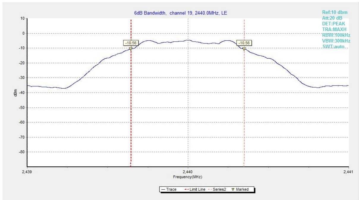
Fig.8 6dB Bandwidth (Ch 19), LE 1M
