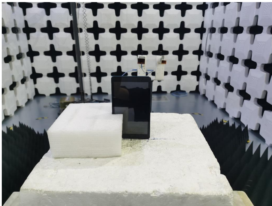
16. Radiated Emissions (Part 15C, 18GHz -26.5GHz)
