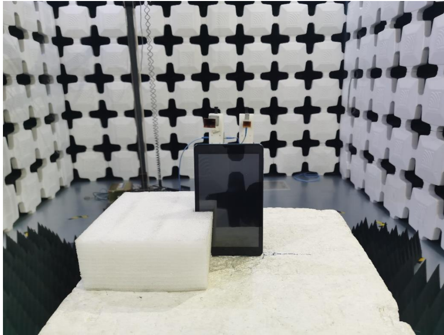
17. Radiated Emissions (Part 15C, 26.5GHz -40GHz)
