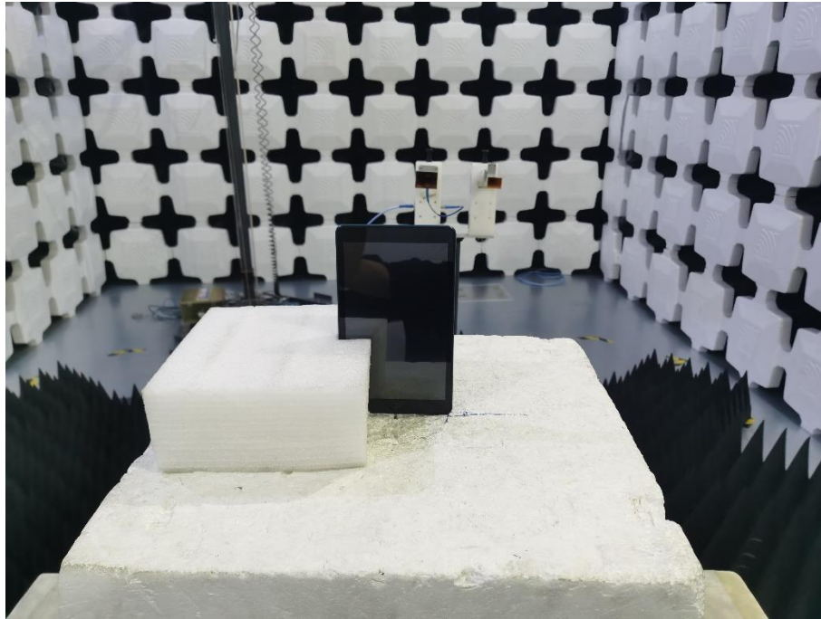
19. Radiated Emissions (Part 22/24/27, 18GHz -26.5GHz)
