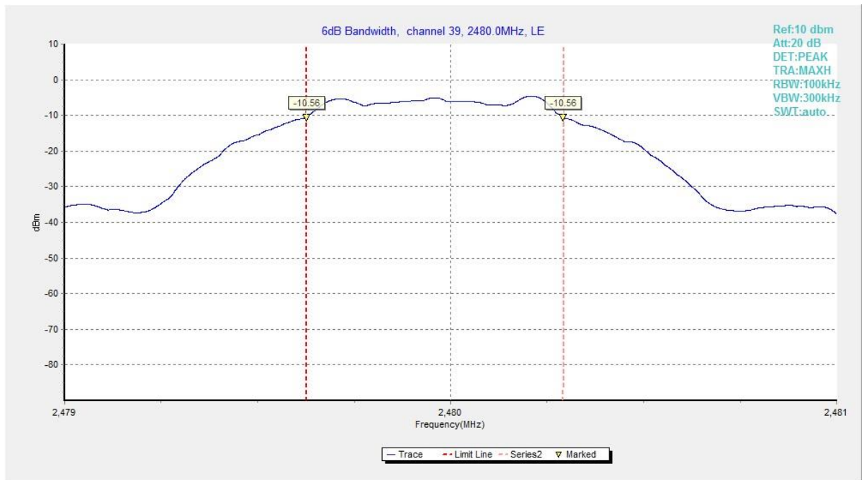
Fig.9 6dB Bandwidth (Ch 39), LE 1M
