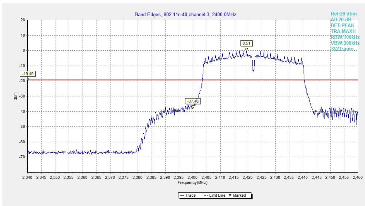
Fig.31 Band Edges (802.11n HT40, CH 3)
