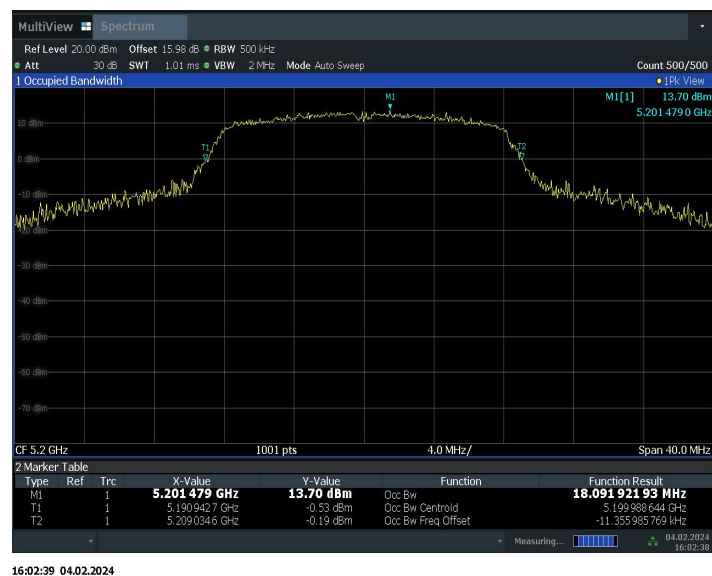
Fig.61 99% Occupied bandwidth (802.11a, 5200MHz)
