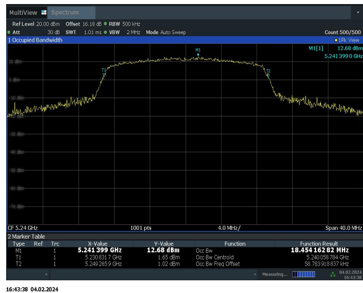
Fig.65 99% Occupied bandwidth (802.11ac-VHT20, 5240MHz)
