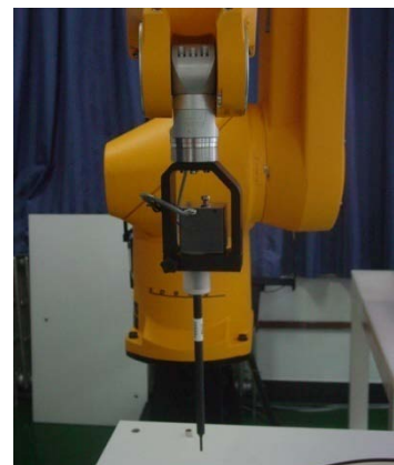
Picture C.3 E-field Probe
