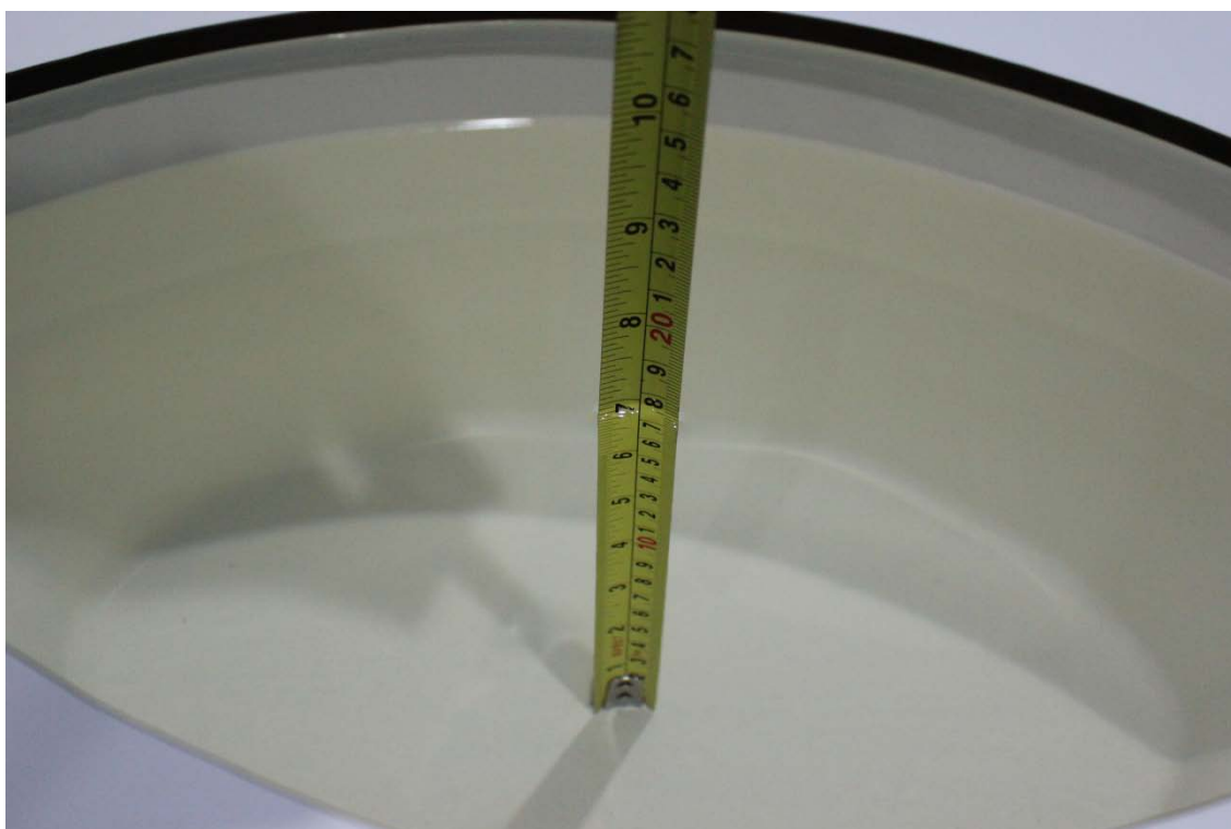
Picture 7-10 Liquid depth in the Flat Phantom (5GHz)
