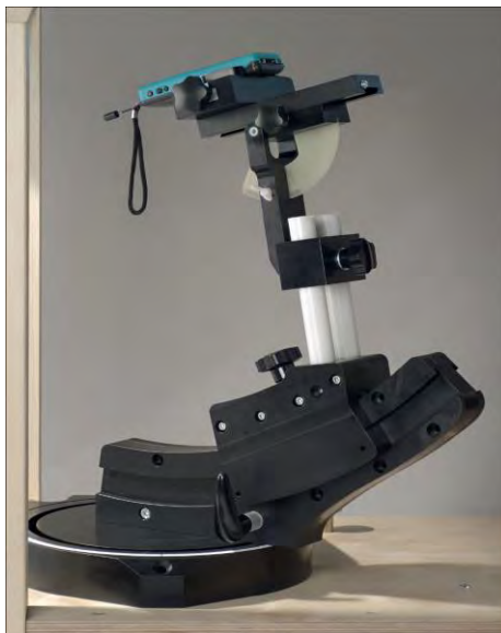
F-2. Device Holder for Transmitters
