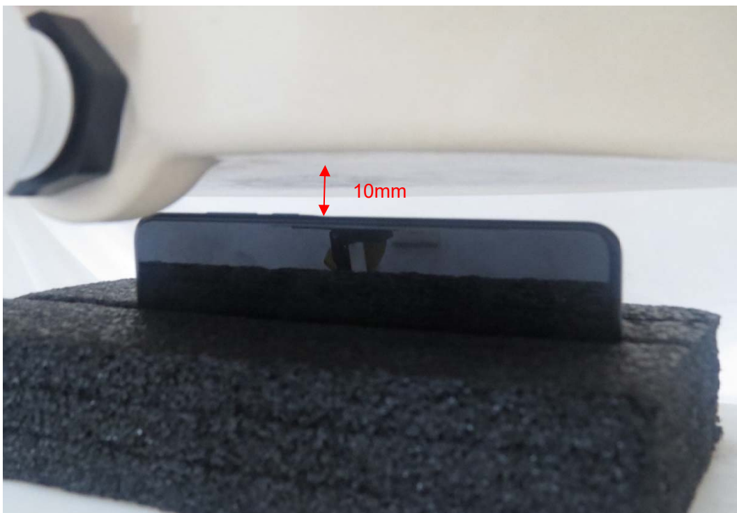
Picture 10: Right Edge, the distance from handset to the bottom of the Phantom is 10mm
