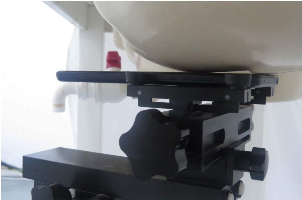
Picture 1: Left Hand Touch Cheek Position
