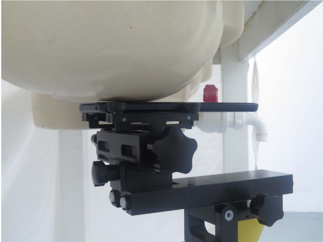
Picture 3: Right Hand Touch Cheek Position
