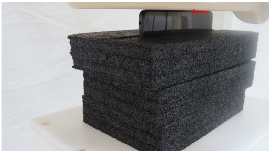
Picture 14: Left Edge, the distance from handset to the bottom of the Phantom is 0mm
