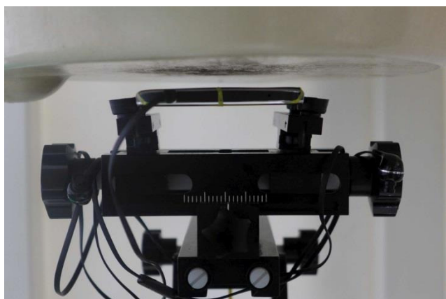
Back with headset, Test Separation 1 cm
