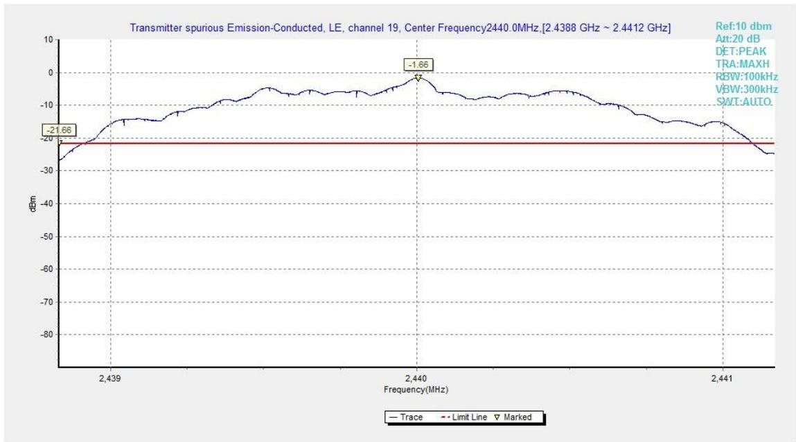
Fig.8. Transmitter Spurious Emission - Conducted: GFSK, 2440MHz
