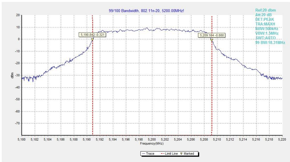
Fig.64 99% Occupied bandwidth (802.11 n-HT20, 5200MHz)
