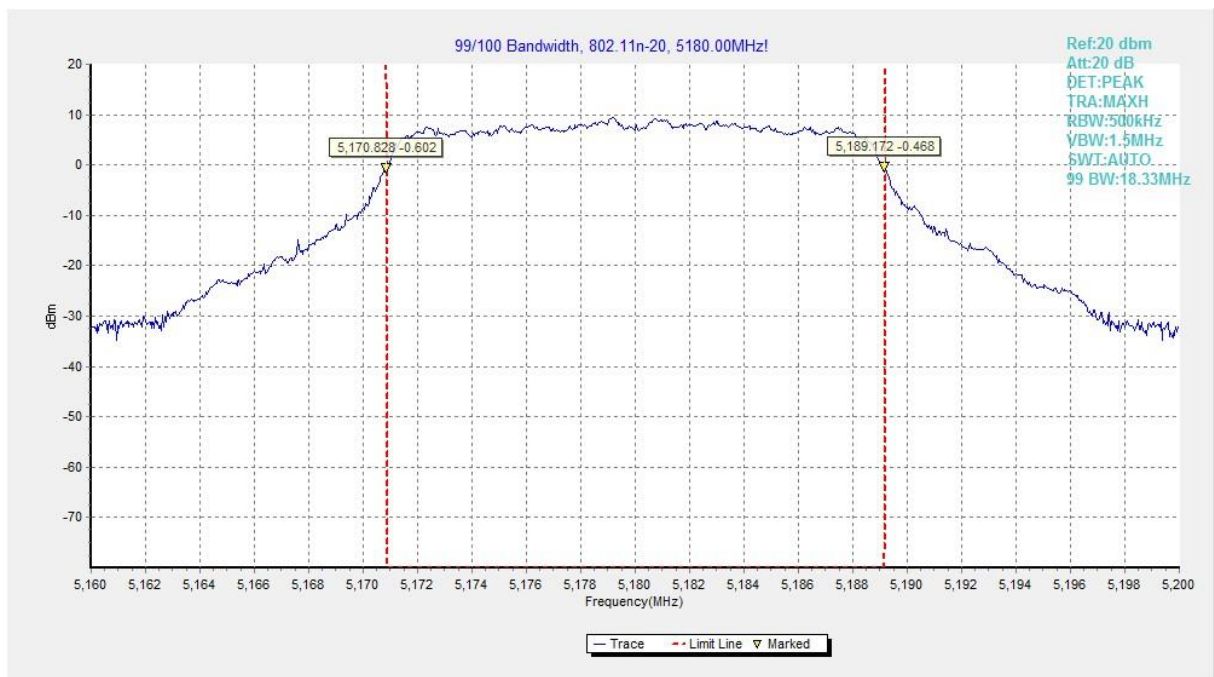
Fig.63 99% Occupied bandwidth (802.11n-HT20, 5180MHz)
