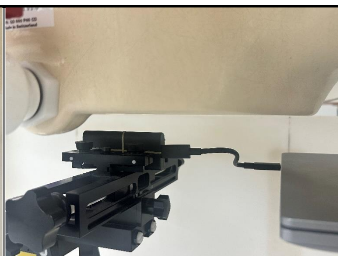
Vertical-Back of EUT with 1.7 cm Gap
