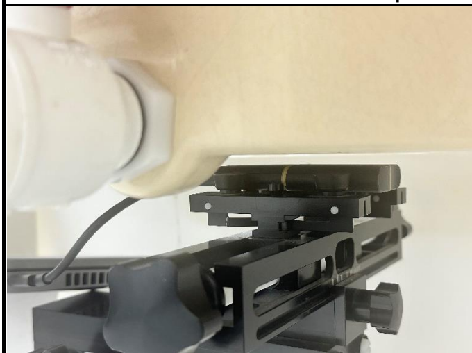
Horizontal-Up of EUT with 0.5 cm Gap
