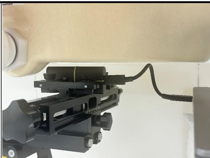
Vertical-Back of EUT with 0.5 cm Gap
