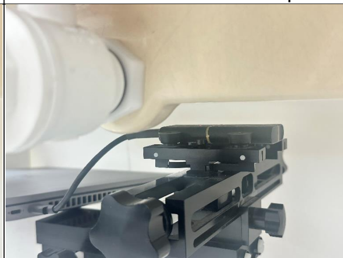
Horizontal-Down of EUT with 1.7 cm Gap
