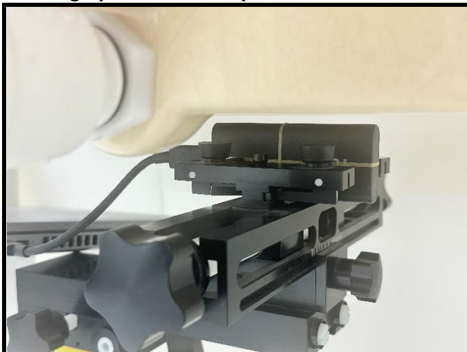
Vertical-Front of EUT with 0.5 cm Gap
