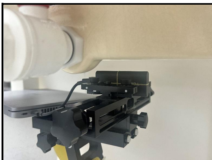
Vertical-Front of EUT with 1.7 cm Gap
