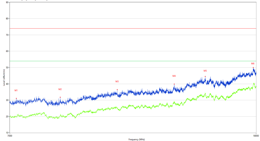
REmission Test case_FCC_Part 15C_FCC 15.247.7GHz-18GHz
