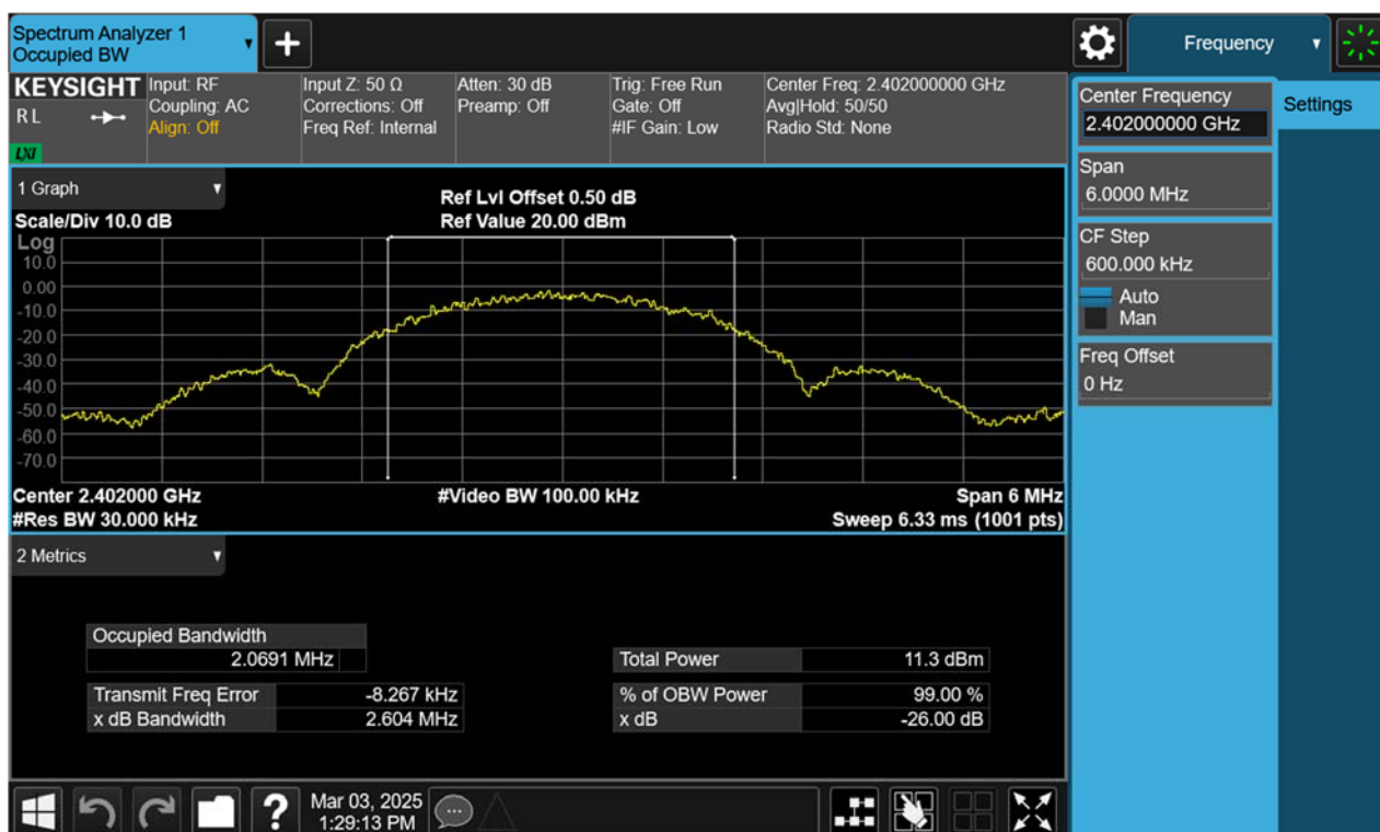
99% Bandwidth, 2402MHz, BLE-2Mbps
