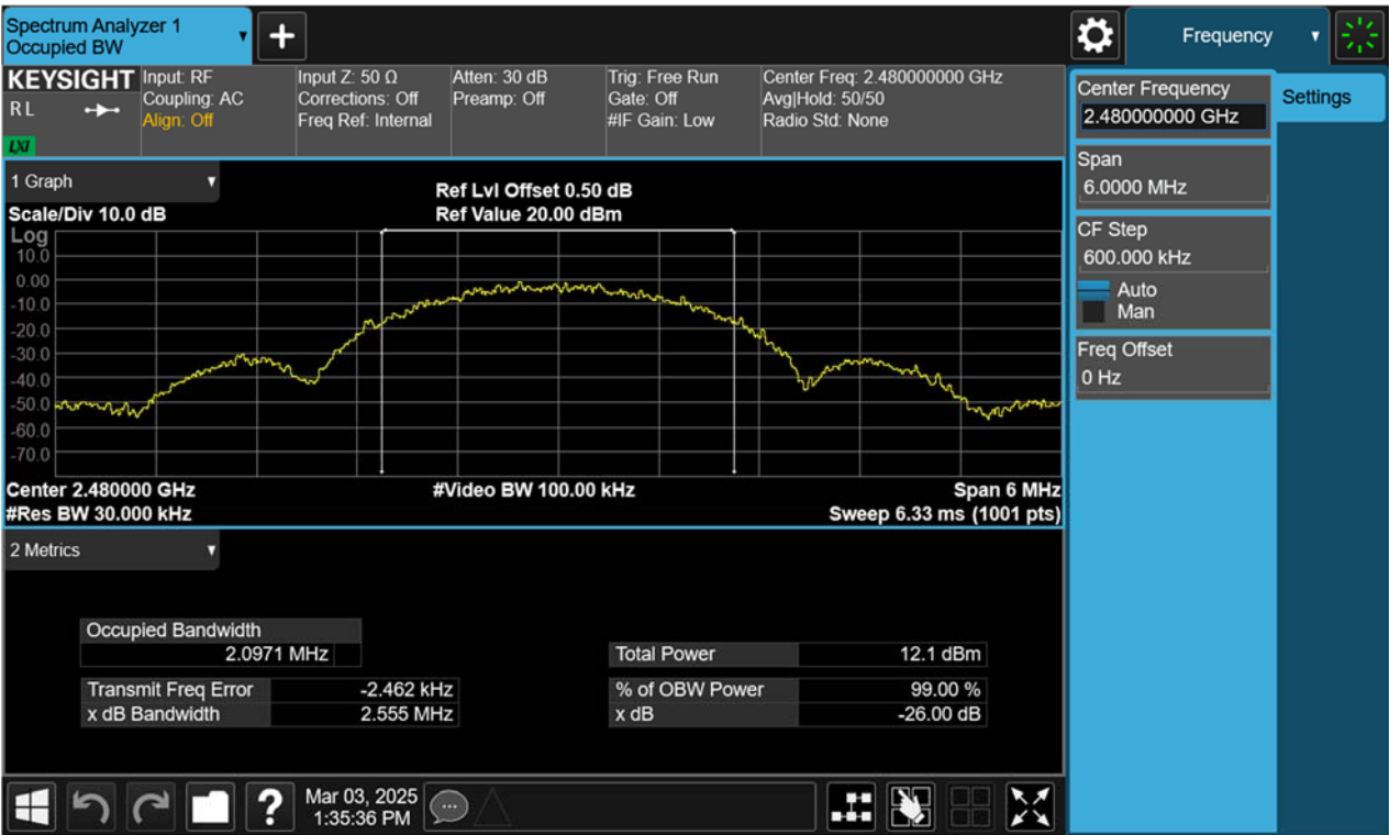
99% Bandwidth, 2480MHz, BLE-2Mbps
