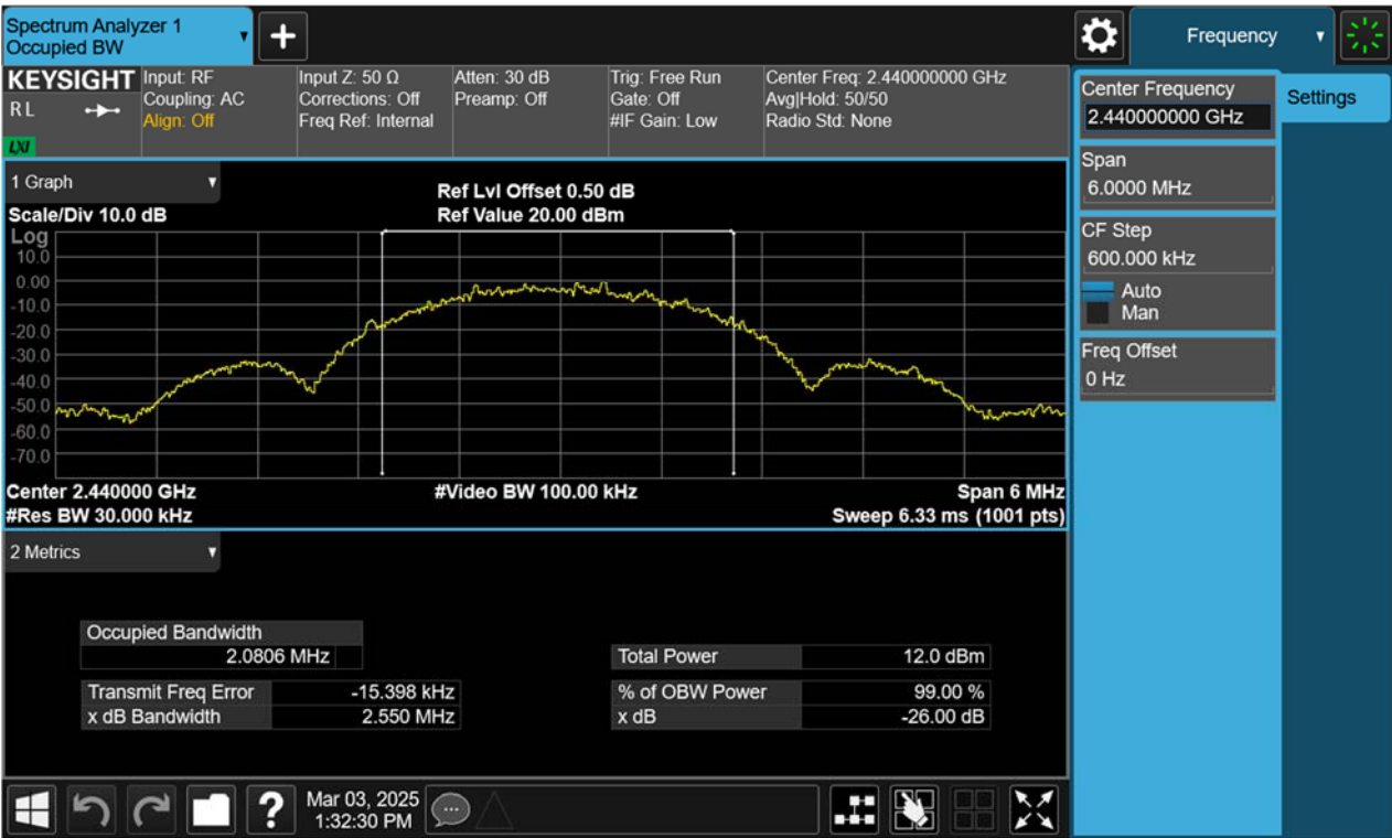
99% Bandwidth, 2440MHz, BLE-2Mbps
