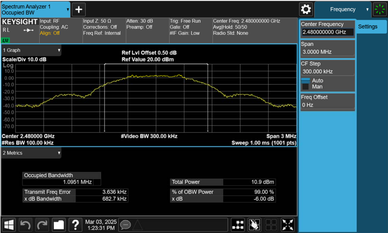
99% Bandwidth, 2480MHz, BLE-1Mbps
