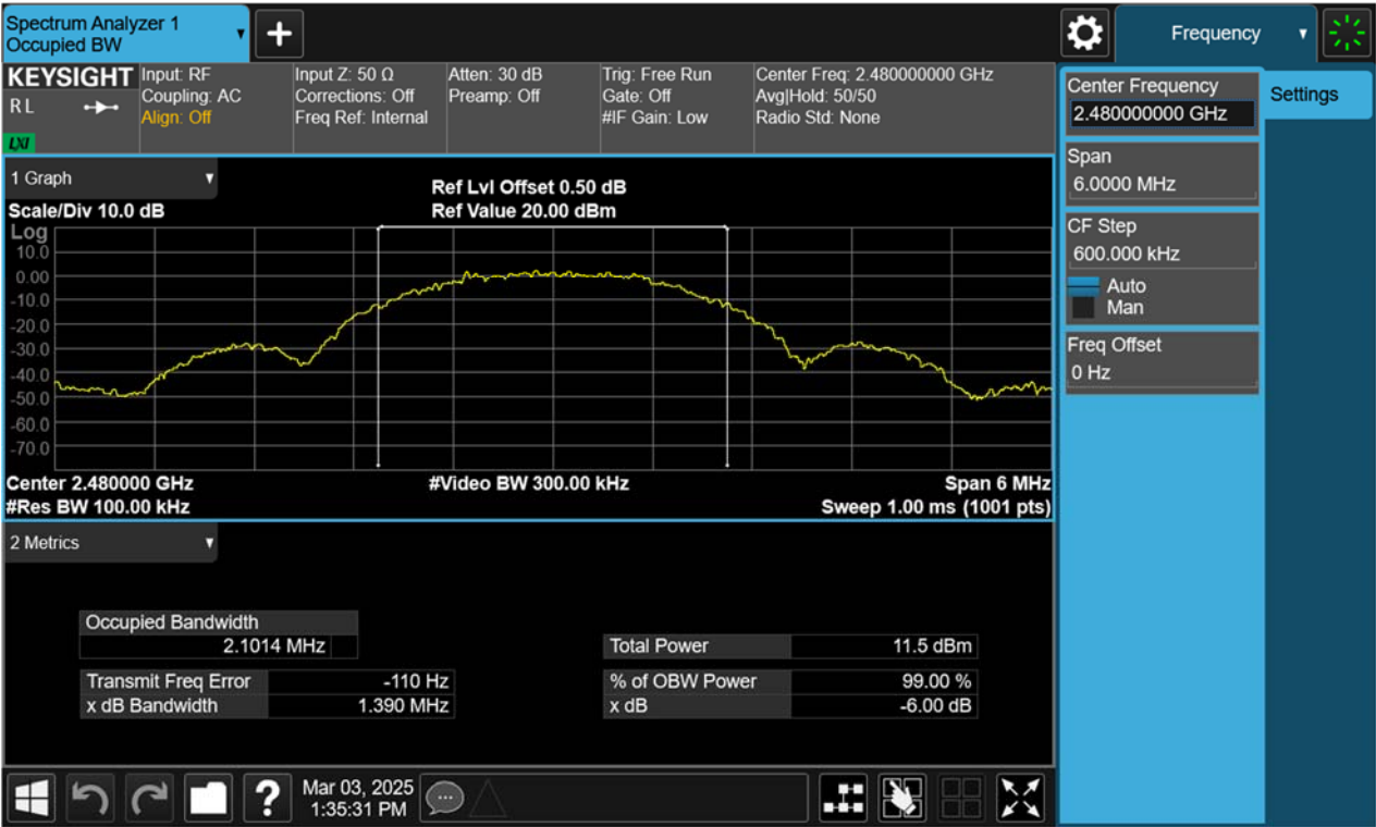
99% Bandwidth, 2480MHz, BLE-2Mbps
