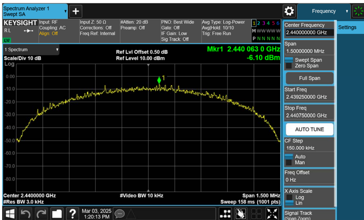
Figure 14: Power Spectral Density, 2440MHz, BLE-1Mbps
