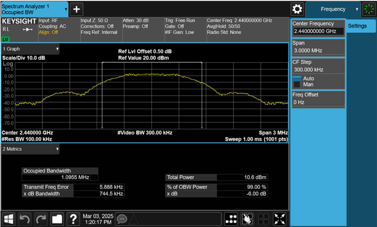
99% Bandwidth, 2440MHz, BLE-1Mbps
