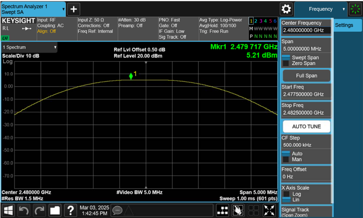
Figure 3: Peak Output Power, 2480MHz, BLE-1Mbps
