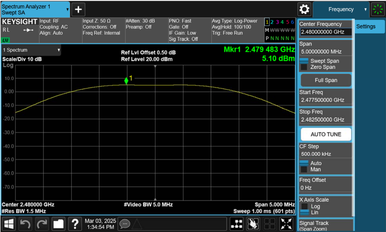
Figure 6: Peak Output Power, 2480MHz, BLE-2Mbps
