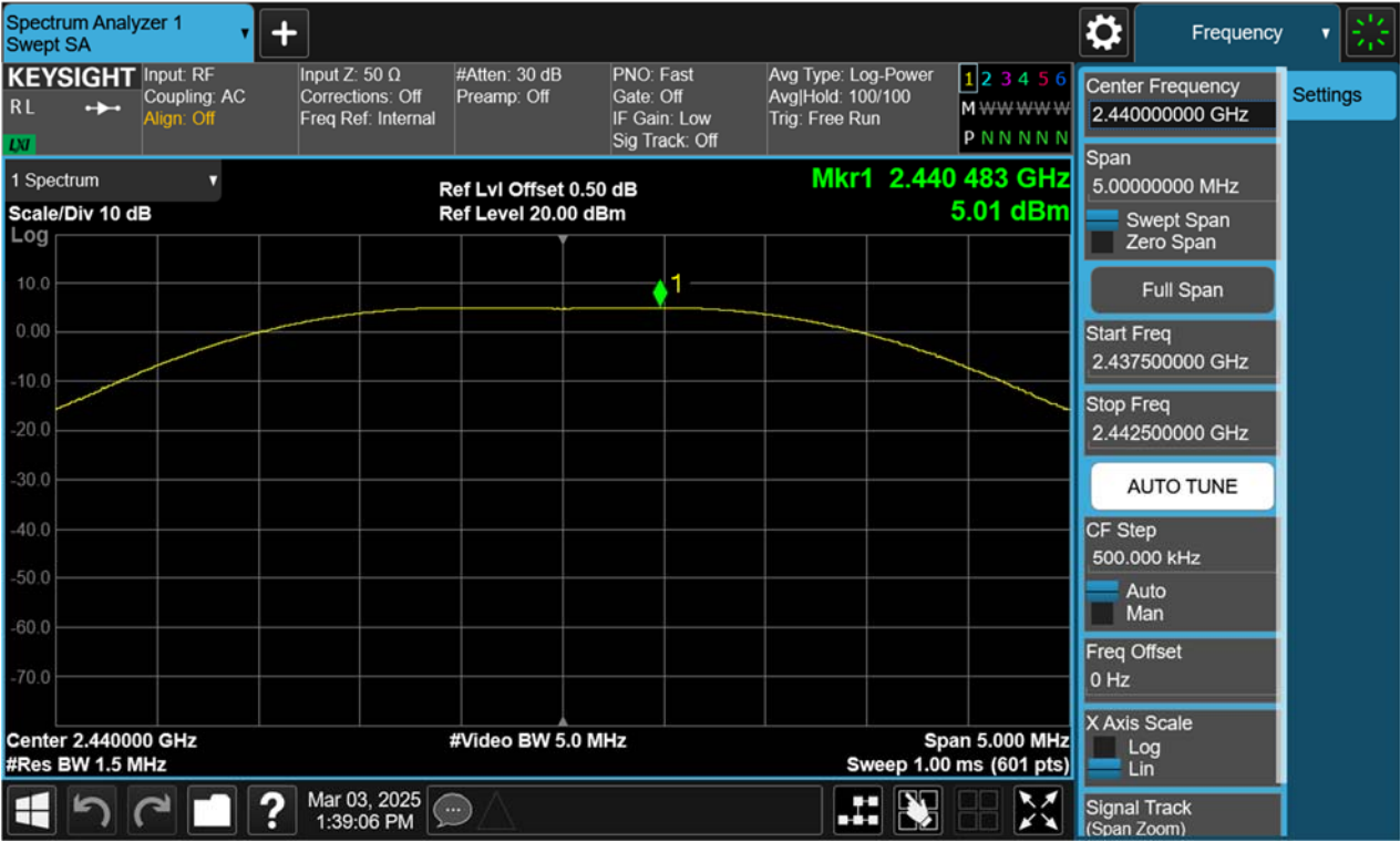
Figure 5: Peak Output Power, 2440MHz, BLE-2Mbps
