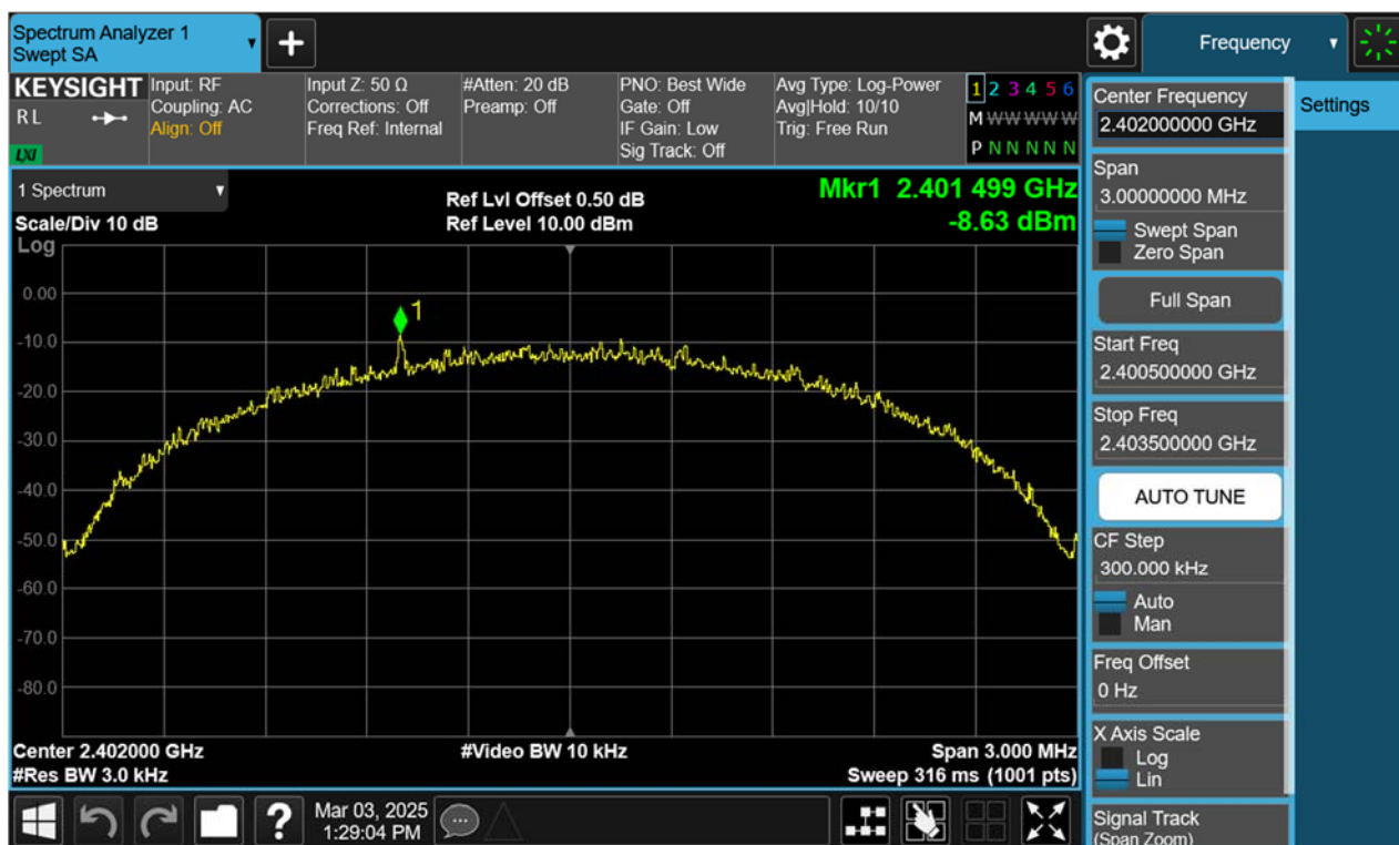
Figure 16: Power Spectral Density, 2402MHz, BLE-2Mbps
