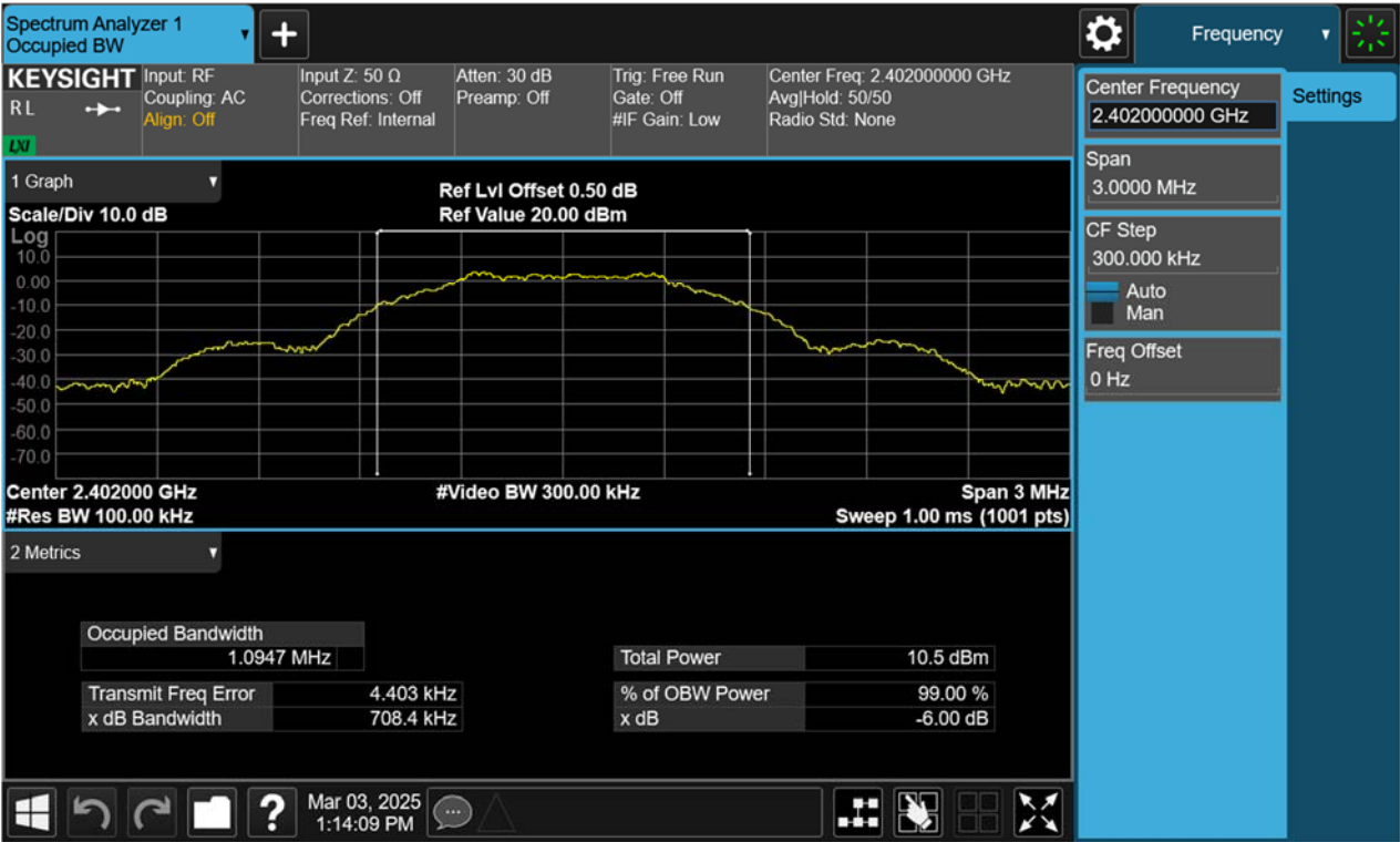
99% Bandwidth, 2402MHz, BLE-1Mbps
