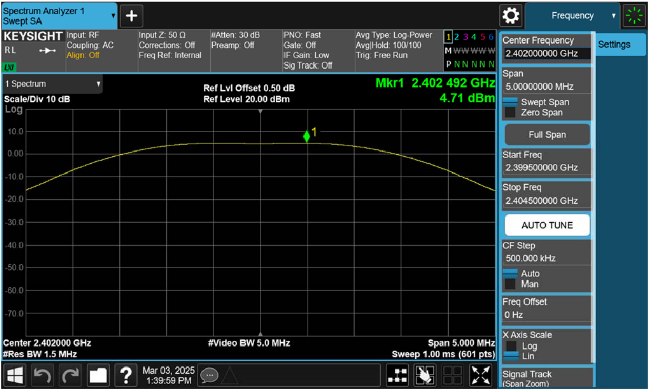
Figure 5: Peak Output Power, 2440MHz, BLE-2Mbps
