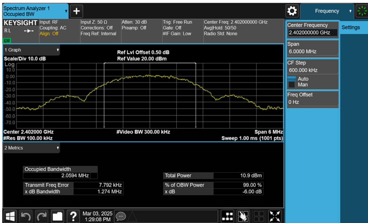
99% Bandwidth, 2402MHz, BLE-2Mbps
