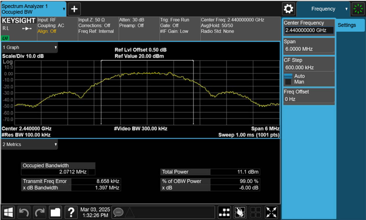
99% Bandwidth, 2440MHz, BLE-2Mbps
