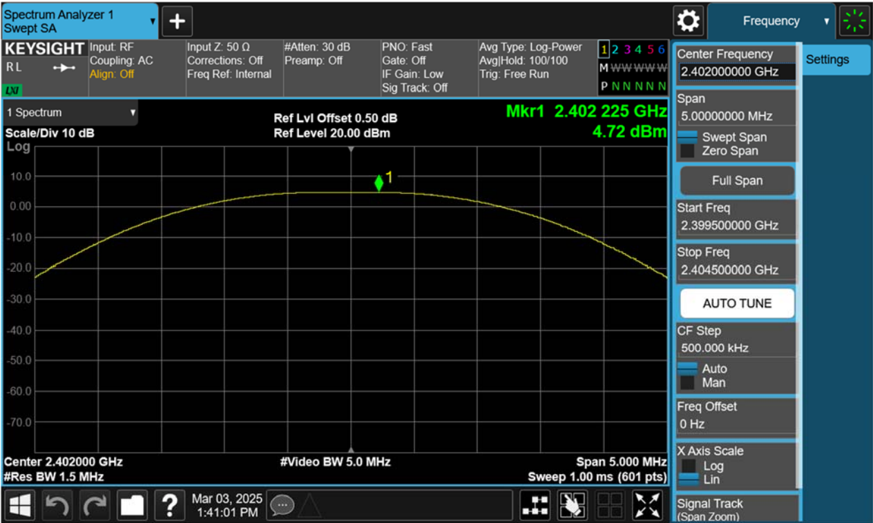
Figure 1: Peak Output Power, 2402MHz, BLE-1Mbps
