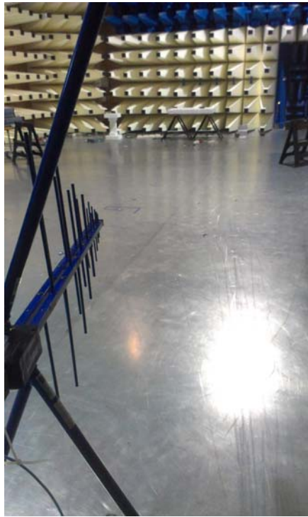
Figure 3: Radiated emissions anechoic chamber 30 MHz to 1 GHz
