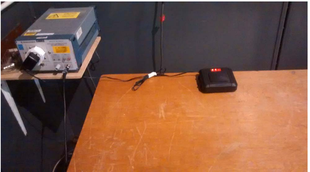
Figure 4: Conducted emissions setup
