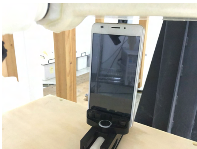
Top of the EUT with 1 cm Gap
