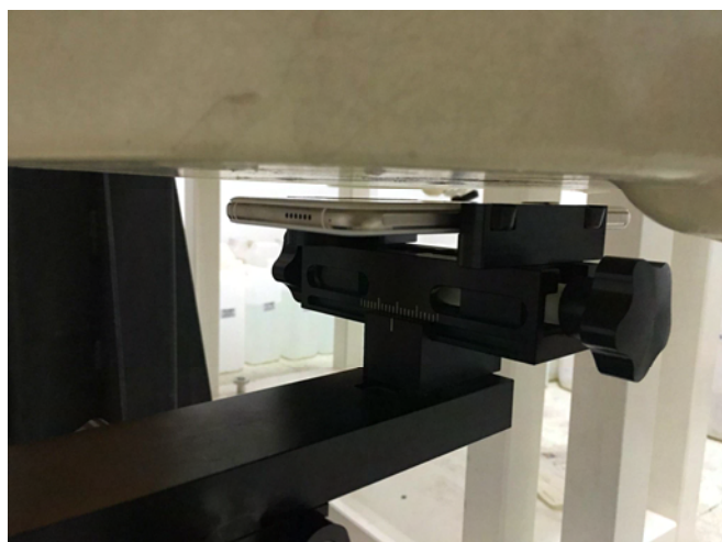
Back of the EUT with 1 cm Gap
